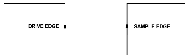
Figure 66. SPI Mode 3, SCLK Edges
