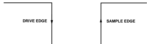
Figure 66. SPI Mode 3, SCLK Edges
