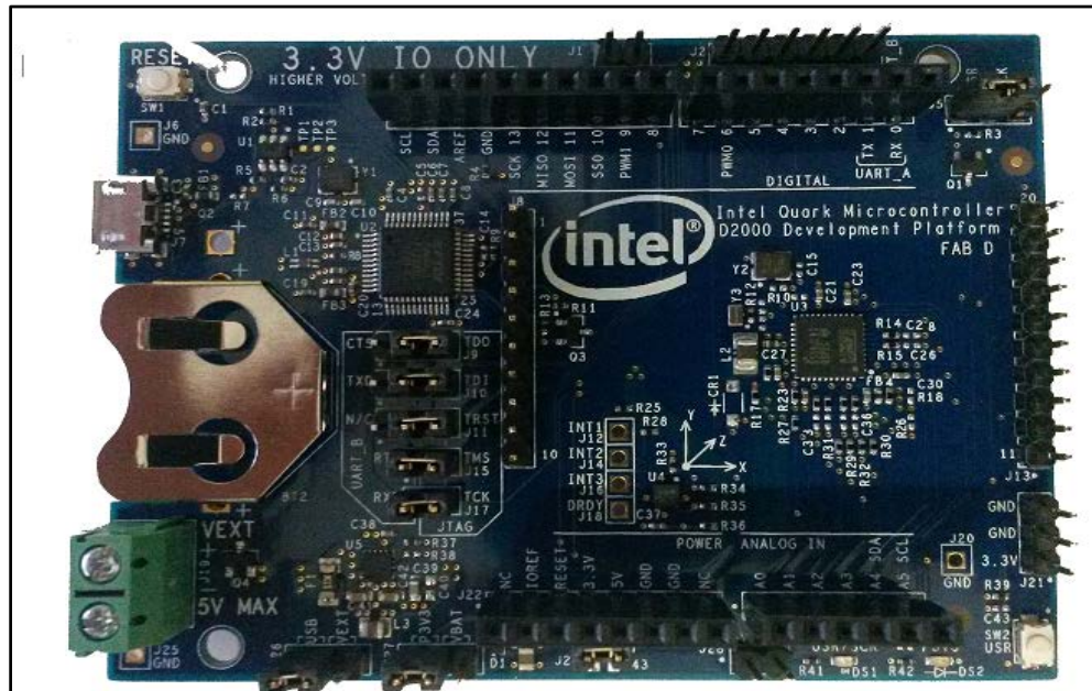
Figure 2. Intel® Quark™ Microcontroller Developer Kit D2000 Fab D Board Photo
