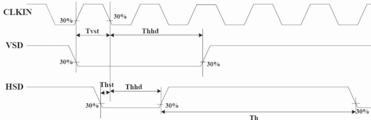
Figure 4: Data Transaction Timing in Parallel RGB (24Bit) interface (SYNC Mode)
