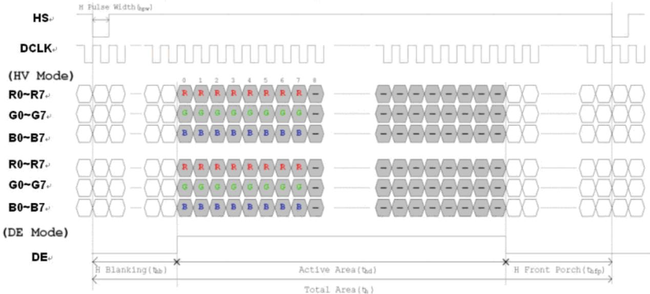
Figure 5: Horizontal Input Timing Diagram
