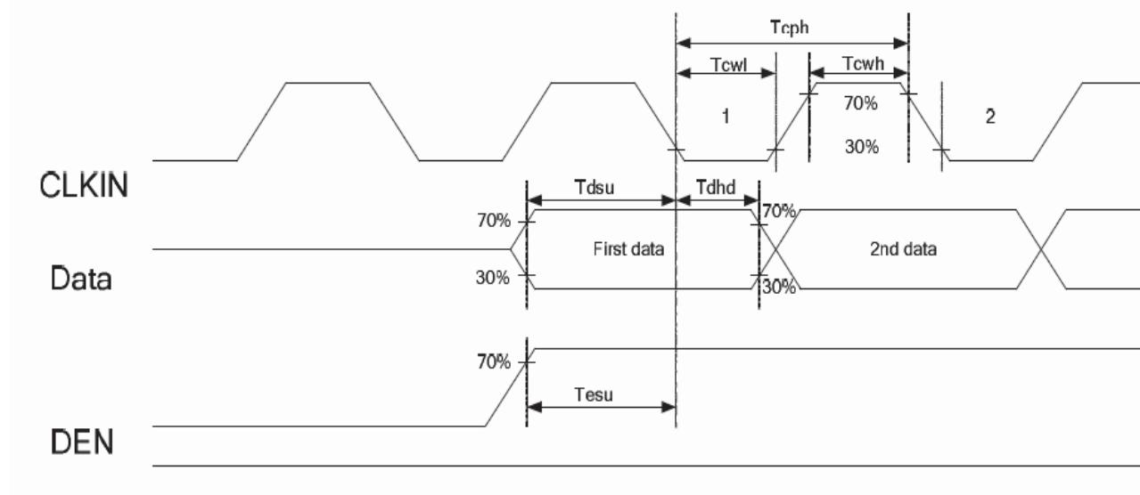
Figure 3: Clock input Data/Den timing diagram
