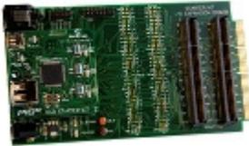
The Microchip PIC32 Accessory Development Starter Kit for Android™ is used for evaluating and developing accessories for Google's Android operating system for smartphones and tablets. It consists of the PIC32 USB Starter Kit, the Starter Kit I/O Expansion Board, and software libraries and APP, available via free download.
