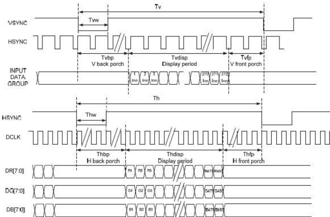
Figure 3:SYNC-DE Mode Timing Diagram
