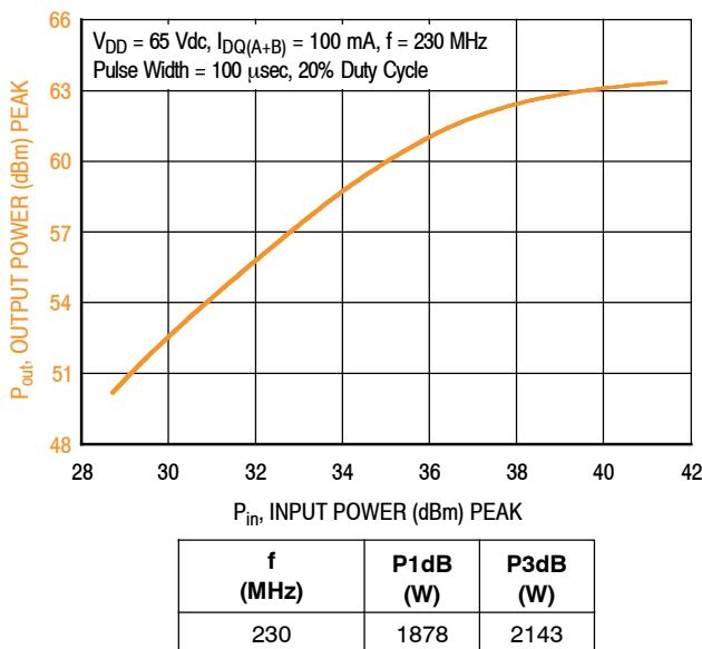
**Figure 13. Output Power versus Input Power**
