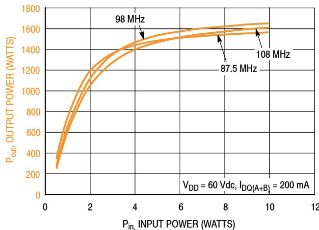
**Figure 7. CW Output Power versus Input Power and Frequency**
