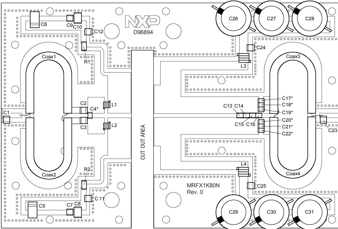
\*C4, C17, C18, C19, C20, C21 and C22 are mounted vertically.
