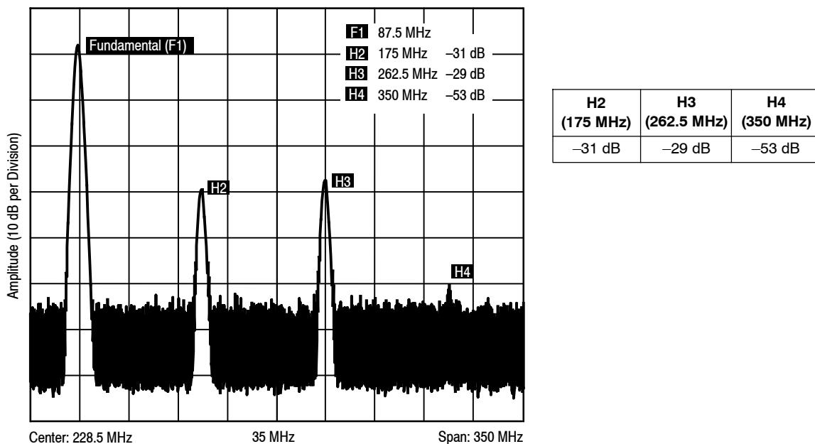
Figure 10. 87.5 MHz Harmonics @ 1500 W CW
