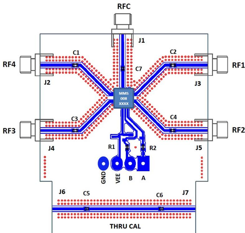
The circuit board used in the application should be generated with proper RF circuit design techniques. Signal lines at the RF port should have 50  $\Omega$  impedance, and the package ground leads and backside ground paddle should be connected directly to the ground plane similar to the previous image.
