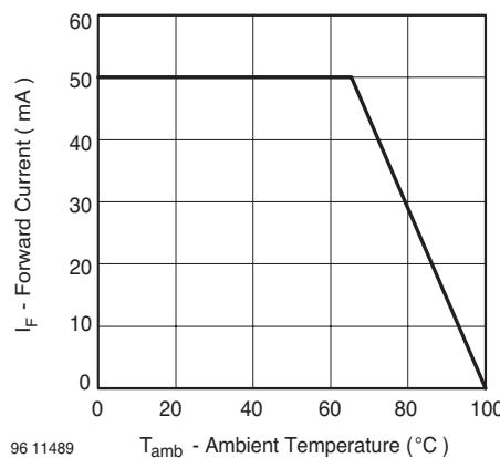
Figure 2. Forward Current vs. Ambient Temperature for AllnGaP
