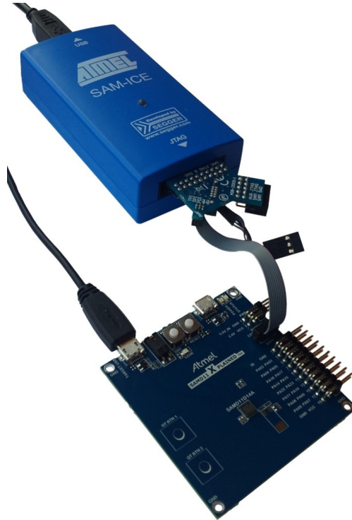
Figure 7-7. SAM-ICE using an Atmel-ICE Adapter
