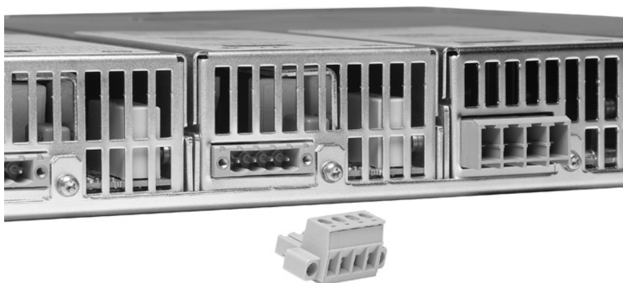
Figure 5. Quick disconnects for power and sense leads
