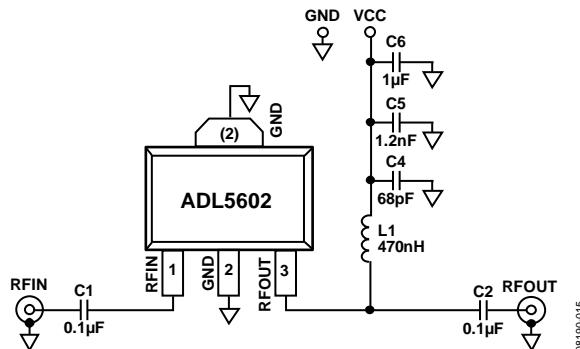
Figure 16. Basic Connections
