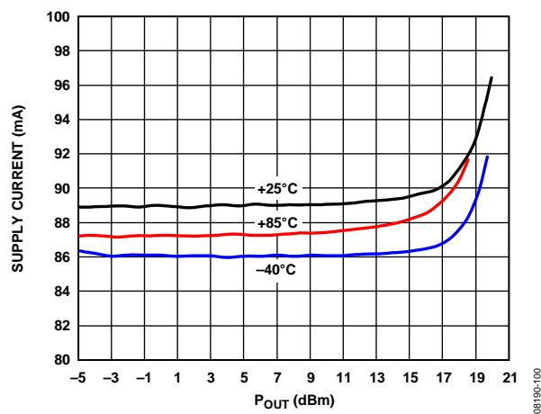
Figure 15. Supply Current vs.  $P_{OUT}$  and Temperature  $V_{CC} = 5\text{ V}$
