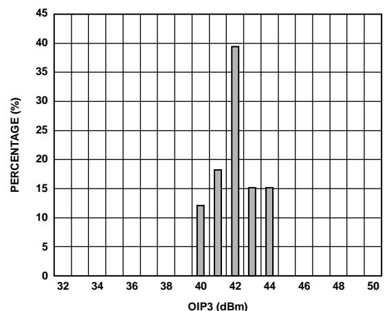
Figure 12. OIP3 Distribution at 2000 MHz,  $P_{out} = 0 \text{ dBm}$
