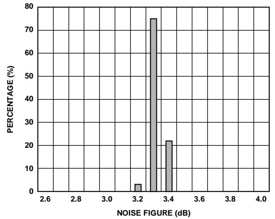
Figure 13. Noise Figure Distribution at 2000 MHz
