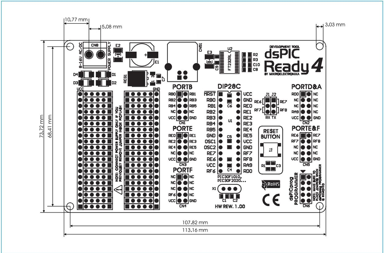
Figure 4: Dimensions of the pločice dsPIC Ready4 additional board
