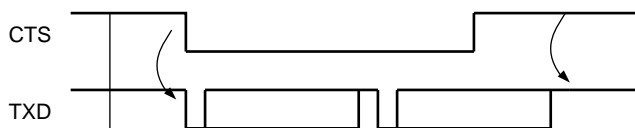
Figure 34-29. Transmitter Behavior when Operating with Hardware Handshaking
