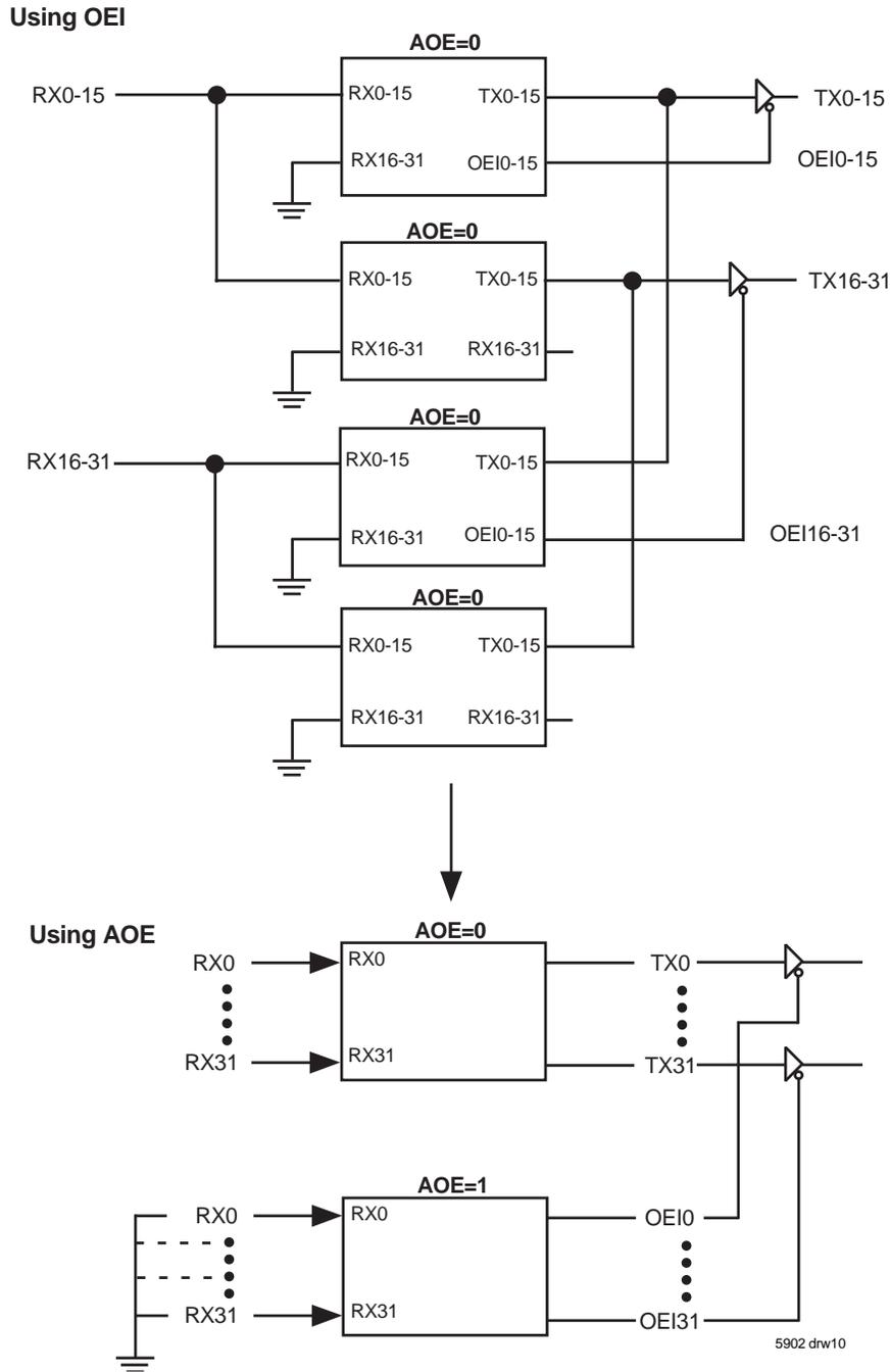
Figure 8. Using All Output Enable (AOE)
