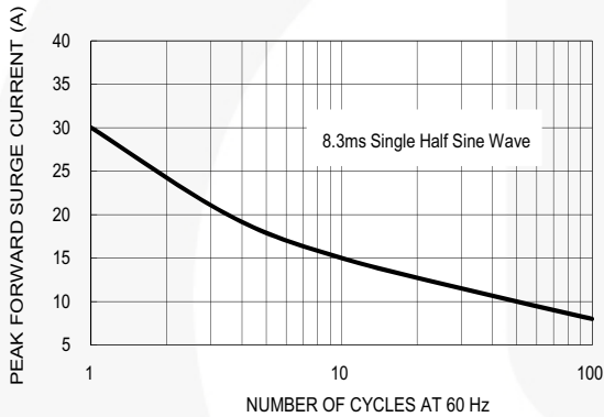
Figure 3. Maximum Non-Repetitive Forward Surge Current
