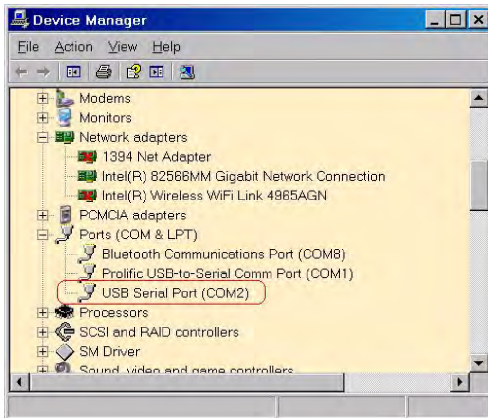
Figure 12. A Successful USB-to-UART Driver Installation
