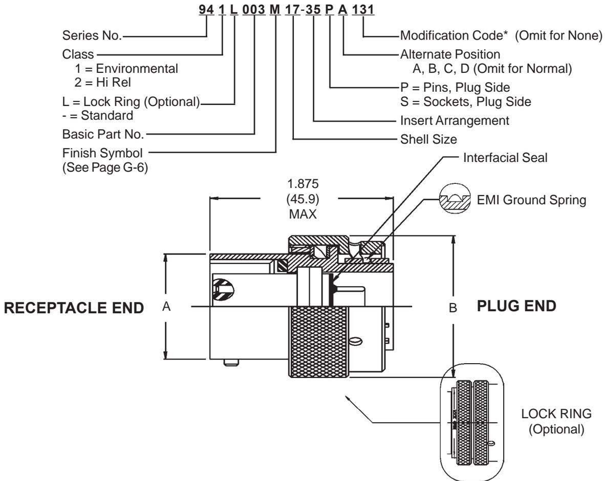
\*Add Modification Code 131 for Dry Lubricant on inside surfaces of Coupling Nut.
