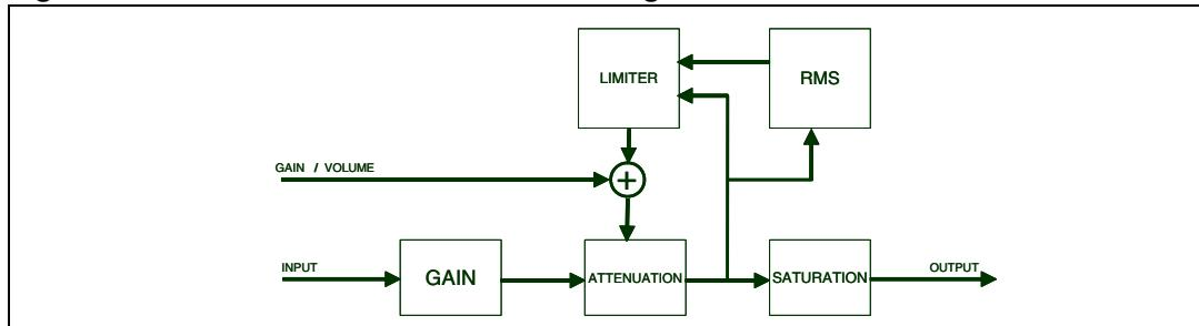
The limiter attack thresholds are determined by the LxAT registers.
