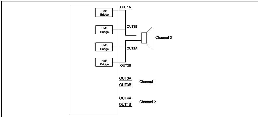
The STA333BW can be configured to support different output configurations. For each PWM output channel a PWM slot is defined. A PWM slot is always  $1 / (8 * fs)$  seconds length. The PWM slot define the maximum extension for PWM rise and fall edge, that is, rising edge as far as the falling edge cannot range outside PWM slot boundaries.
