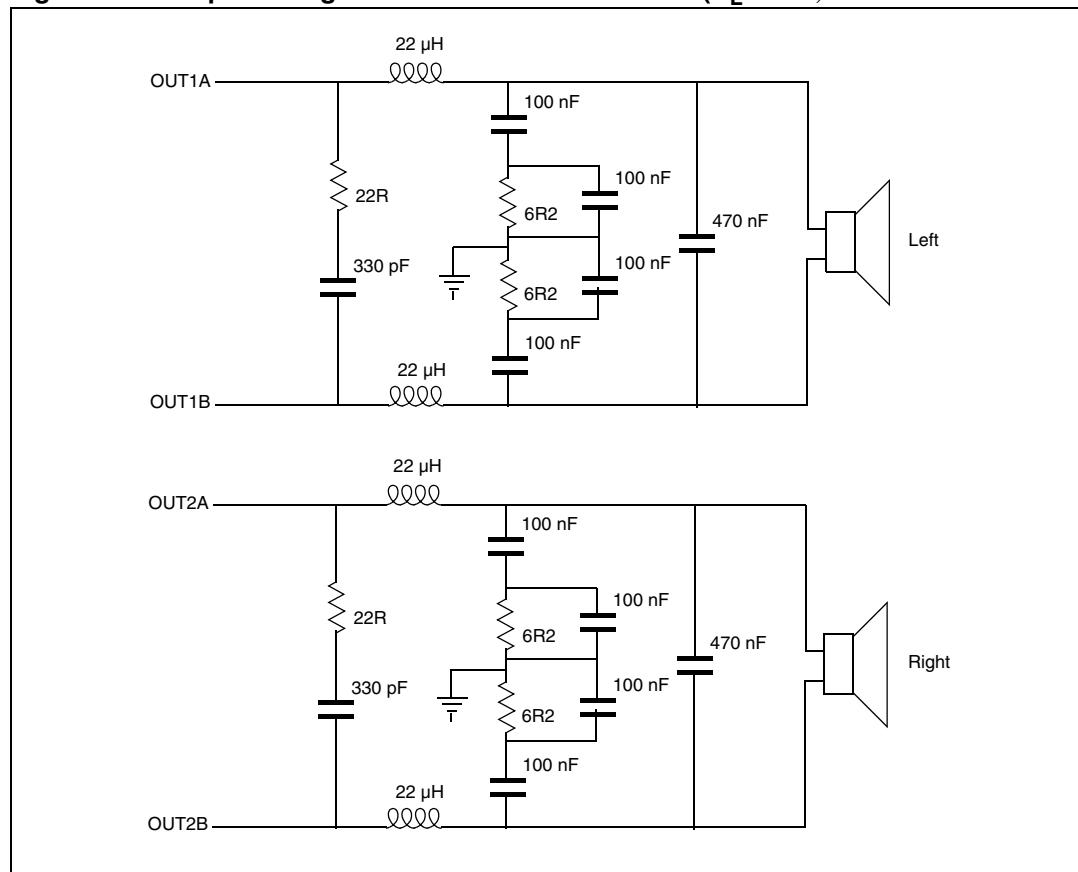
Figure 20. Applications circuit
