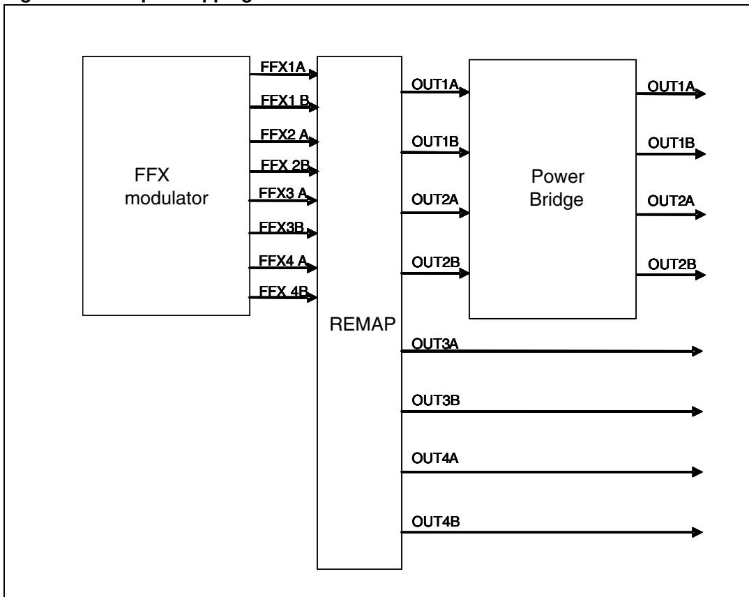
For each configuration the PWM signals from the digital driver are mapped in different ways to the power stage:
