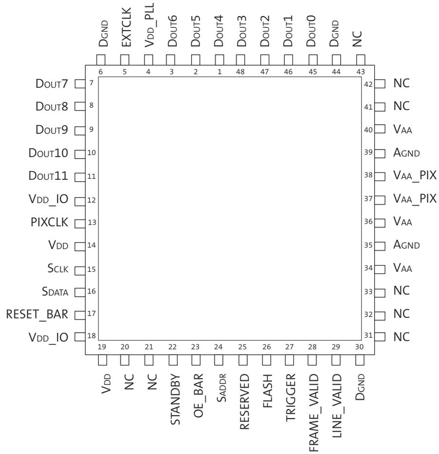
Figure 4: 48-Pin PLCC Pinout Diagram
