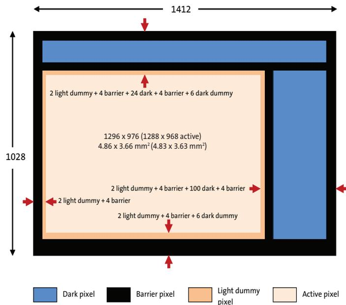
**Figure 6: Pixel Color Pattern Detail (Top Right Corner)**
