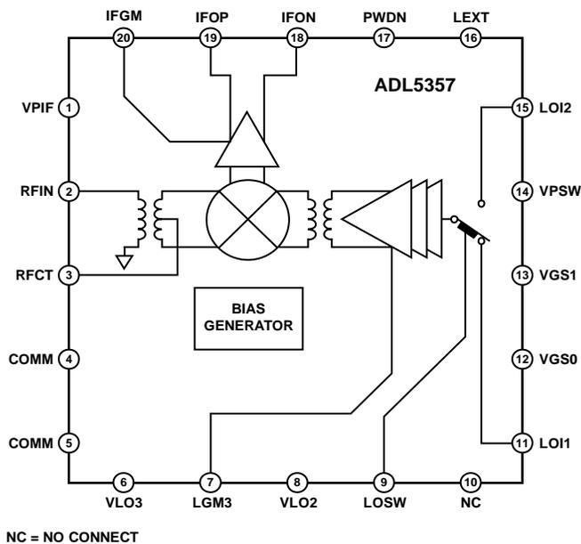
Figure 50. Simplified Schematic
