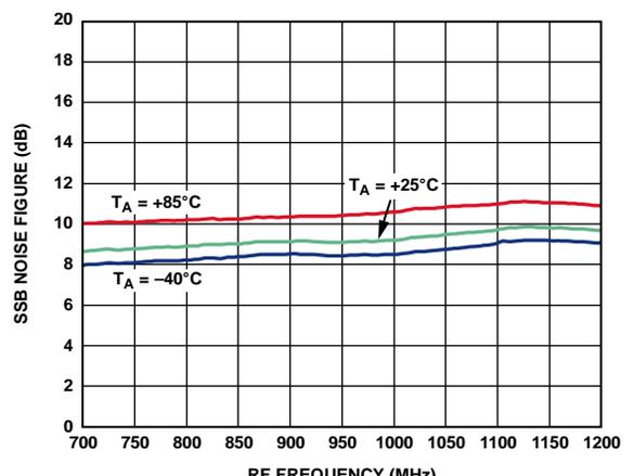
Figure 8. SSB Noise Figure vs. RF Frequency
