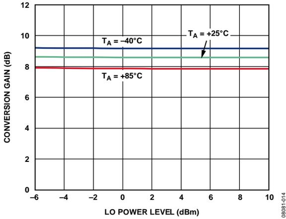
Figure 21. Power Conversion Gain vs. LO Power
