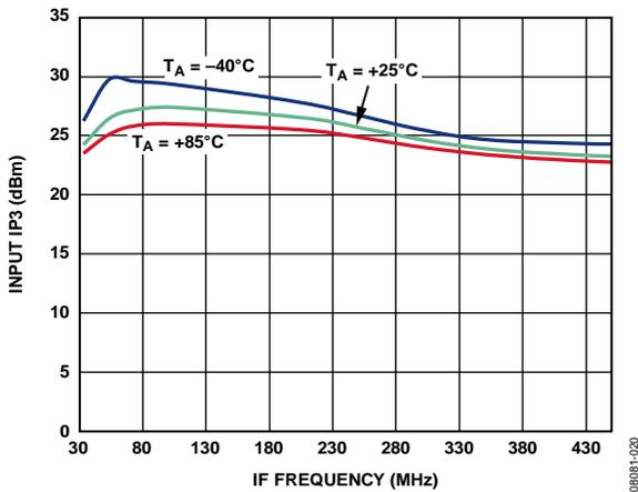
Figure 17. Input IP3 vs. IF Frequency
