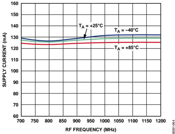
Figure 44. Supply Current vs. RF Frequency at 3.3 V
