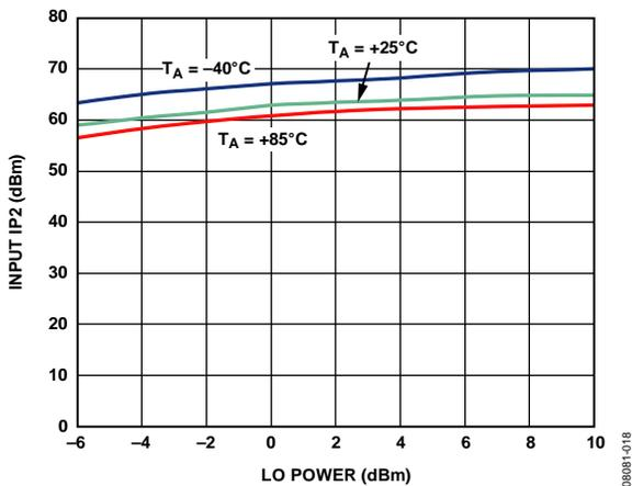
Figure 23. Input IP2 vs. LO Power
