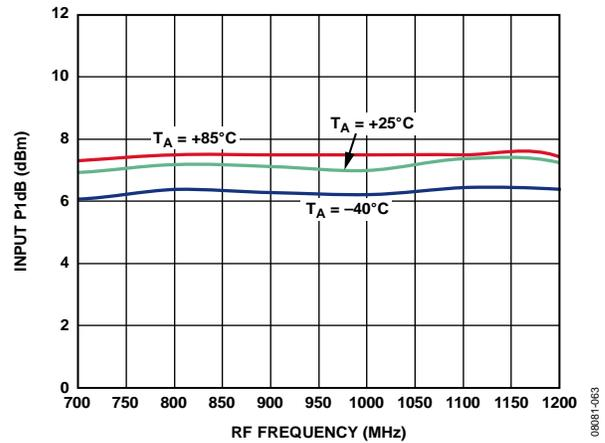
Figure 48. Input P1dB vs. RF Frequency at 3.3 V
