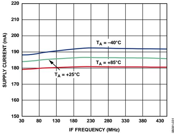
Figure 15. Supply Current vs. IF Frequency
