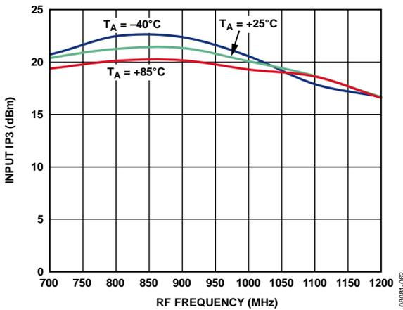
Figure 46. Input IP3 vs. RF Frequency at 3.3 V
