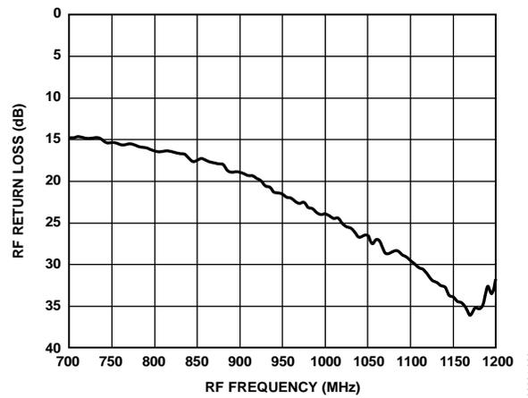
Figure 31. RF Port Return Loss, Fixed IF
