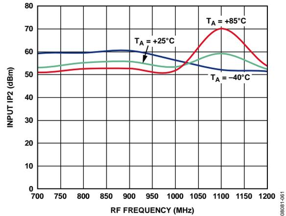
Figure 47. Input IP2 vs. RF Frequency at 3.3 V
