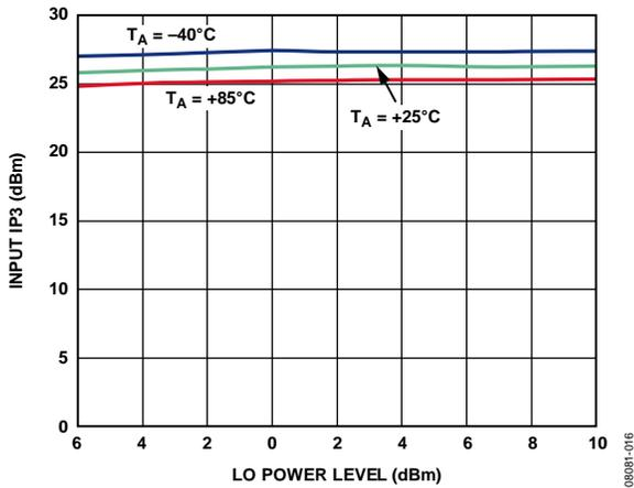
Figure 22. Input IP3 vs. LO Power
