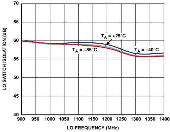
Figure 33. LO Switch Isolation vs. LO Frequency
