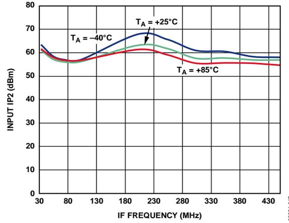
Figure 18. Input IP2 vs. IF Frequency
