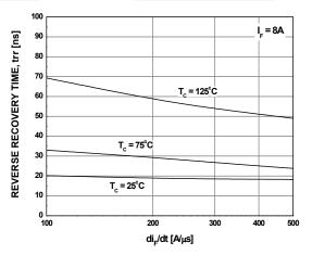
Figure 7. Typical Reverse Recovery Current
