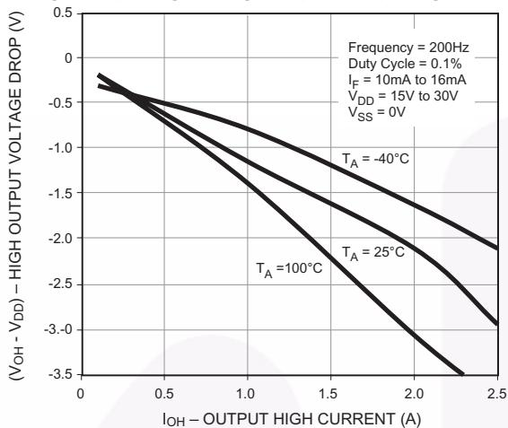
**Fig. 2 Output High Voltage Drop vs. Ambient Temperature**
