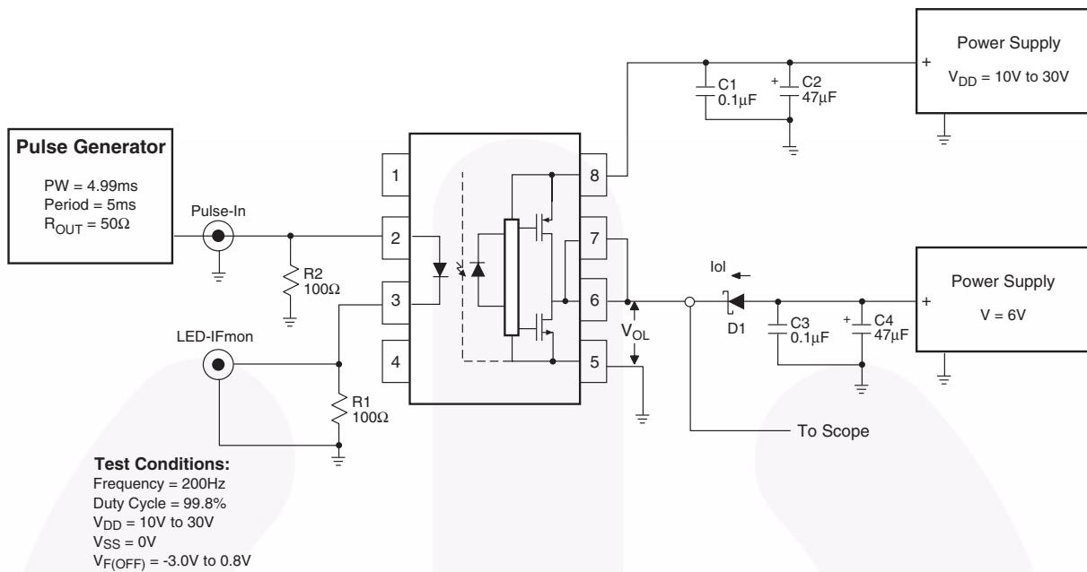
Figure 20. I<sub>OL</sub> Test Circuit
