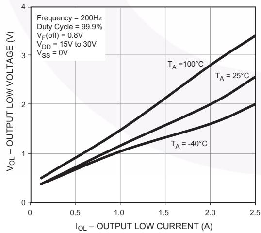
**Fig. 6 Output Low Voltage vs. Ambient Temperature**
