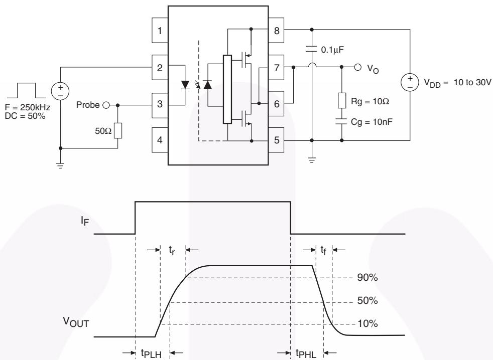
Figure 29.  $t_{PHL}$ ,  $t_{PLH}$ ,  $t_r$  and  $t_f$  Test Circuit and Waveforms
