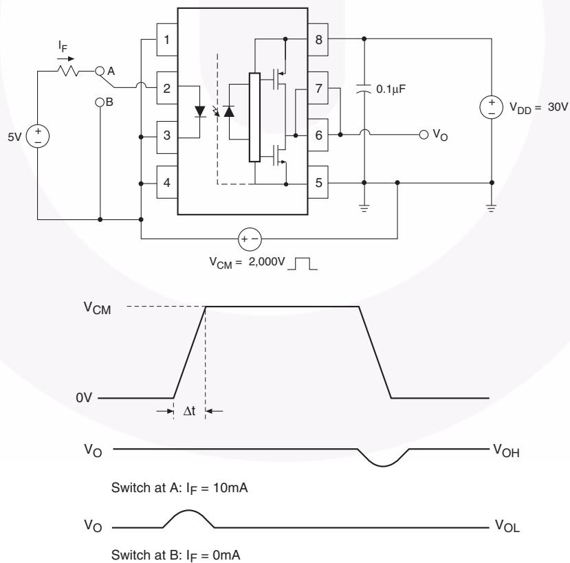
Figure 30. CMR Test Circuit and Waveforms
