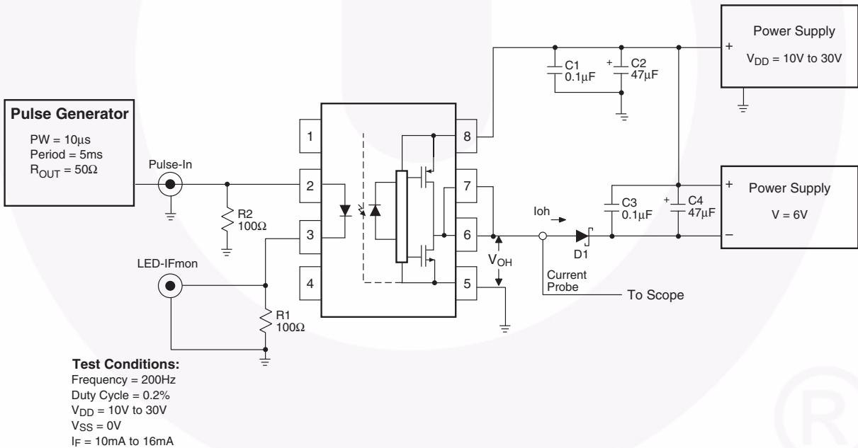
Figure 21. I<sub>OH</sub> Test Circuit
