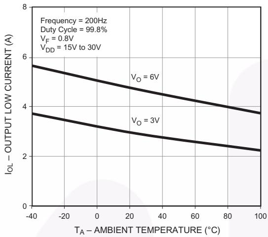
**Fig. 8 Output Low Current vs. Ambient Temperature**
