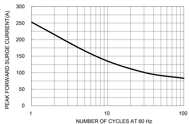
FIG. 3- MAXIMUM NON-REPETITIVE FORWARD SURGE CURRENT
