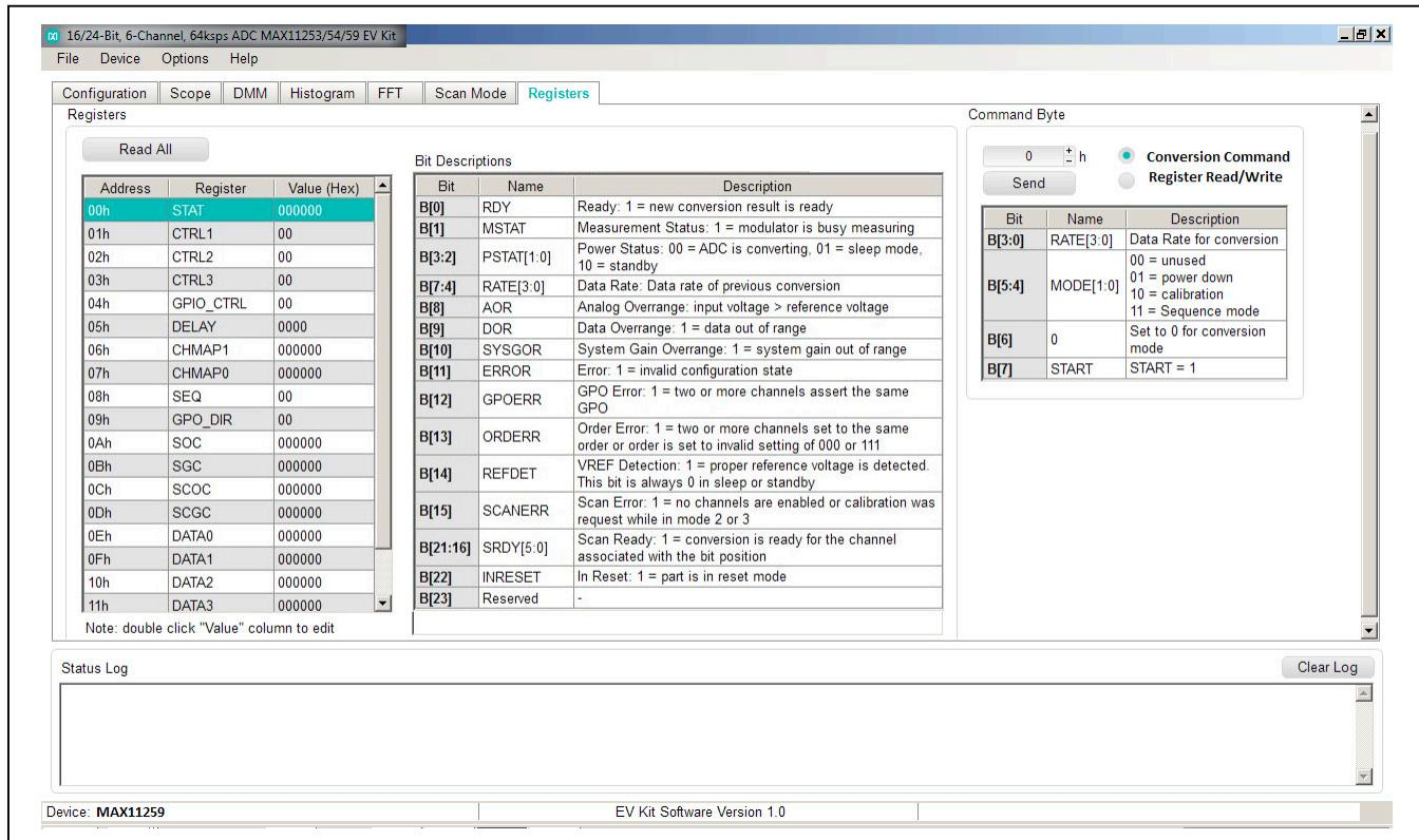
*Figure 8. Peripheral Module Software (ADC Registers Tab)*
