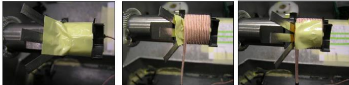
Insert piece of tape after the insulation of N2-N3. Wind N1b. Refold tape, block and connect the wires to pin
