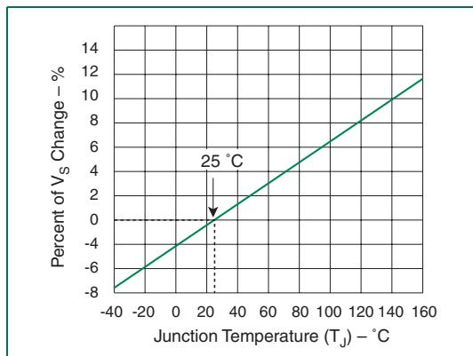
Normalized V<sub>S</sub> Change versus Junction Temperature
