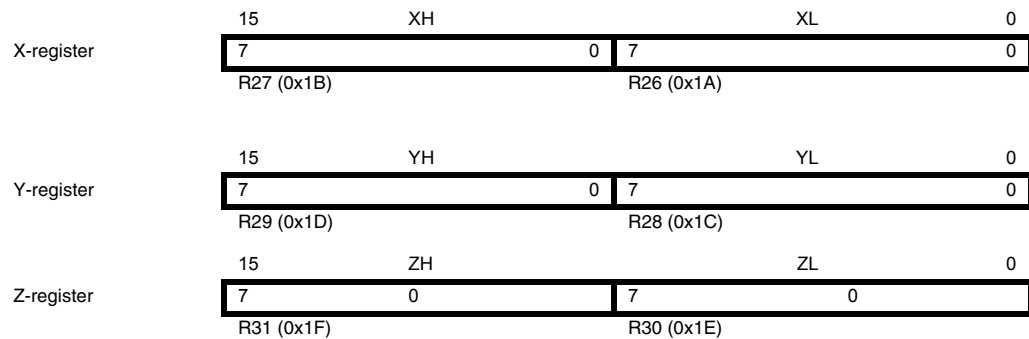
Figure 7-3. The X-, Y-, and Z-registers
