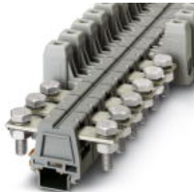
Universal terminal block with screw connection, cross section: 25 - 50 mm 2 , AWG: 6 - 1/0, width: 32 mm, color: gray
