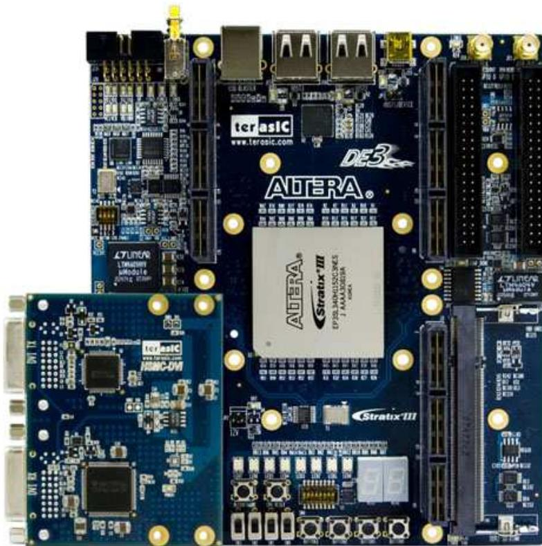
Figure 1.3.2 The HSMC-DVI board connects with DE3
