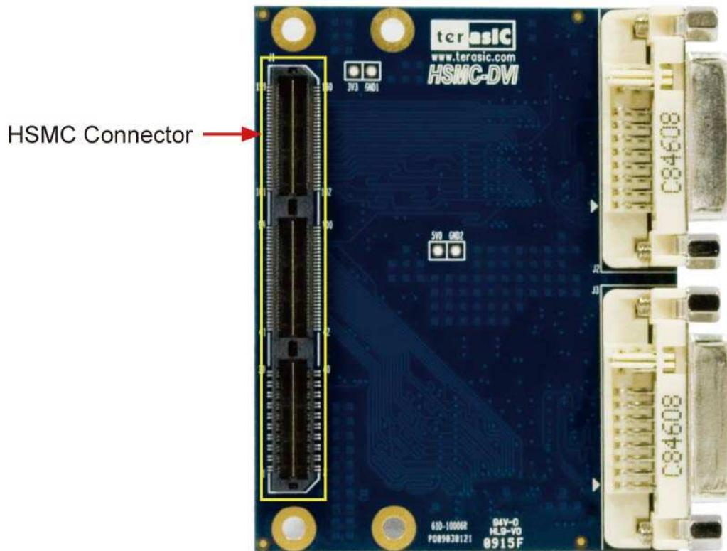
Figure 2.1.2 The HSMC-DVI Back side – HSMC connector view
