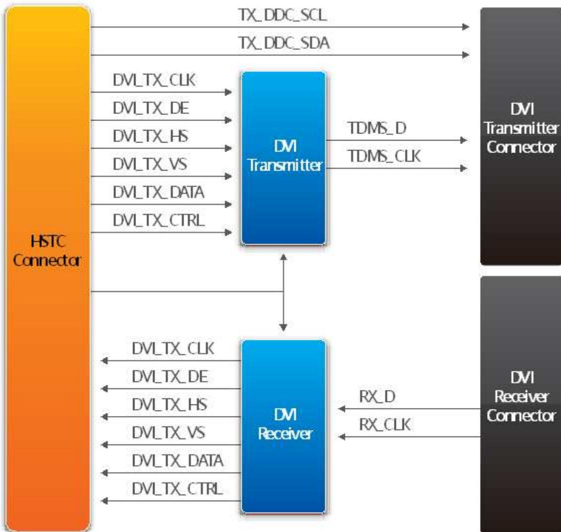
Figure 2.2.1 The block diagram of the HSMC-DVI board
