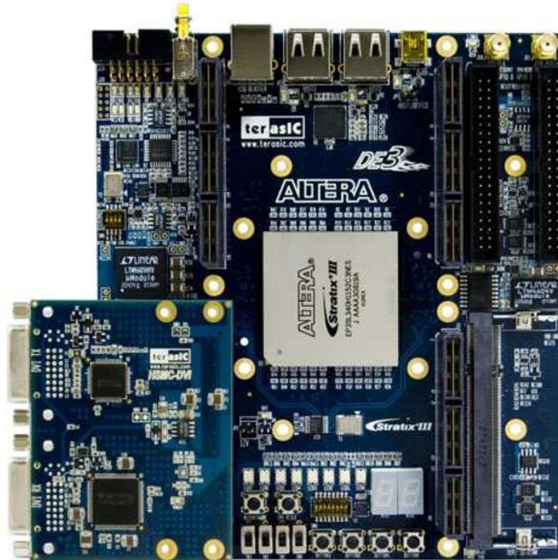
Figure 1.2.1 The HSMC-DVI board connects with DE3
