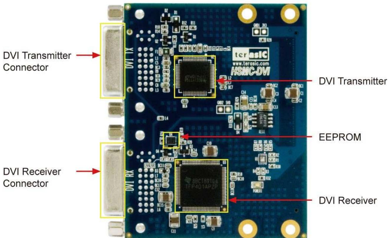
Figure 2.1.1 The HSMC-DVI PCB and component diagram
