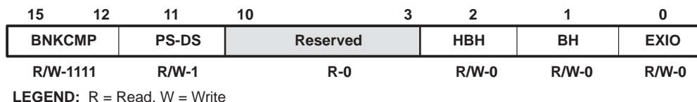
Figure 6. Bank-Switching Control Register (BSCR), MMR Address 0029h
