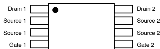
Figure 3. Pinouts for Dual-Die TSSOP
