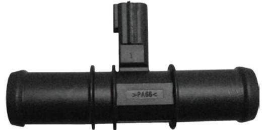
The inline flow-through temperature sensor monitors the temperature of a fluid that passes through it. A system control module receives this temperature reading and uses a control loop to control the overall system temperature. This could be engine temperature, heater temperature, industrial supply temperature, etc.
