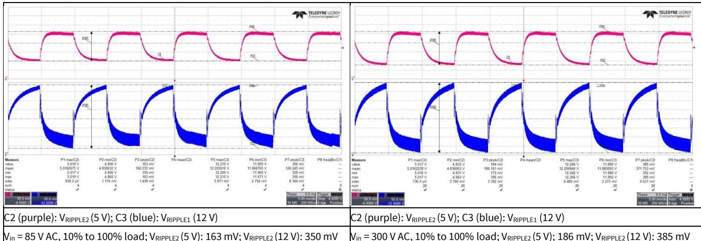
Figure 20 Load transient response
