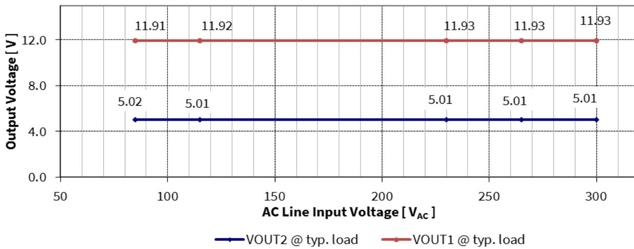
**Line Regulation: Output voltage vs AC line input voltage @ min. load**
