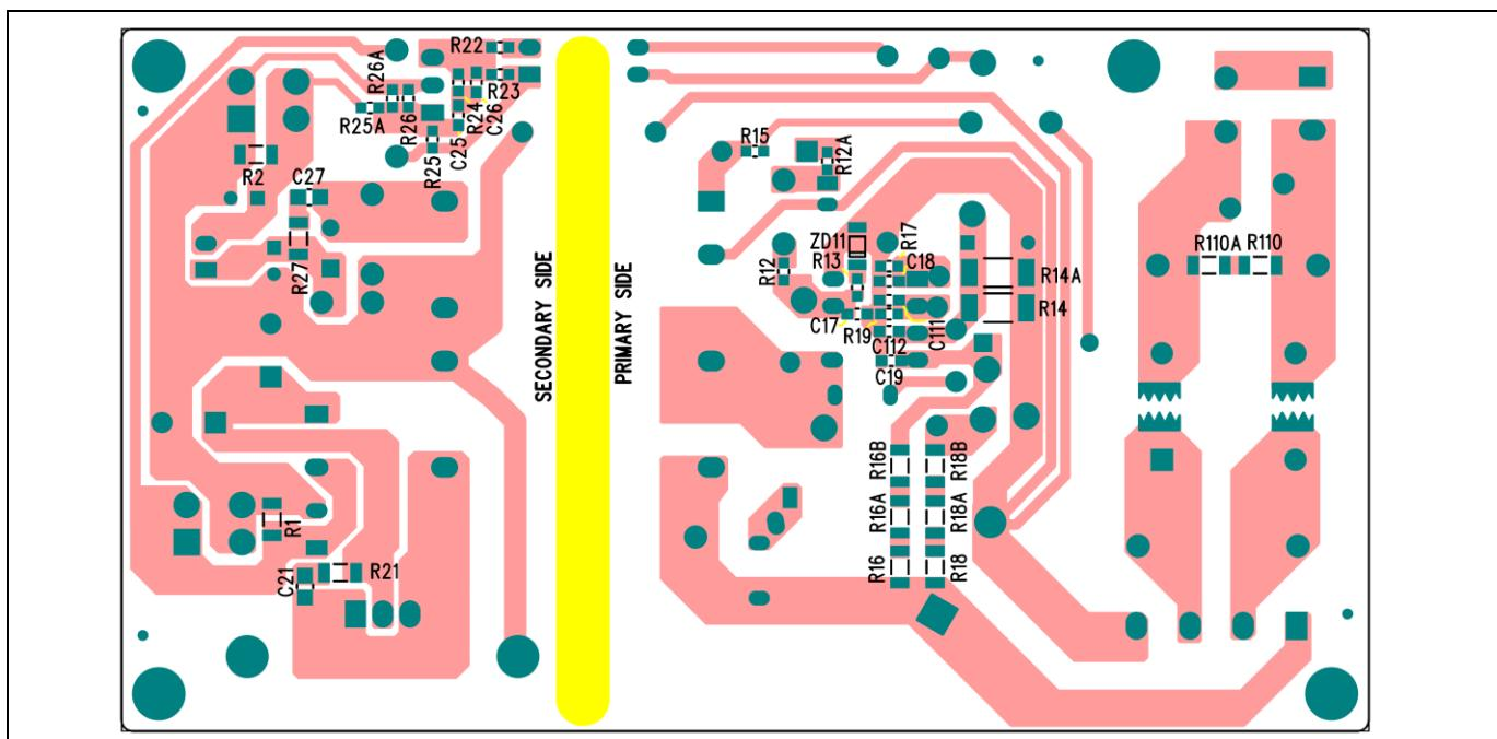
Figure 7 Bottom side copper and component legend
