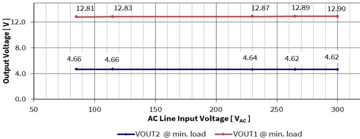
**Figure 10 Line regulation:  $V_{OUT}$  vs AC-line input voltage**
