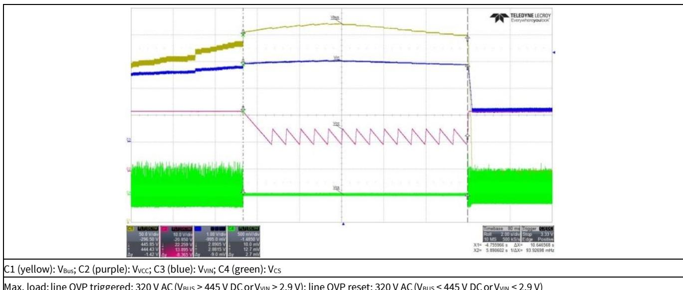
**Figure 21 Line OVP****11.8 Brown-in/Brown-out protection (non-switch auto restart)**
