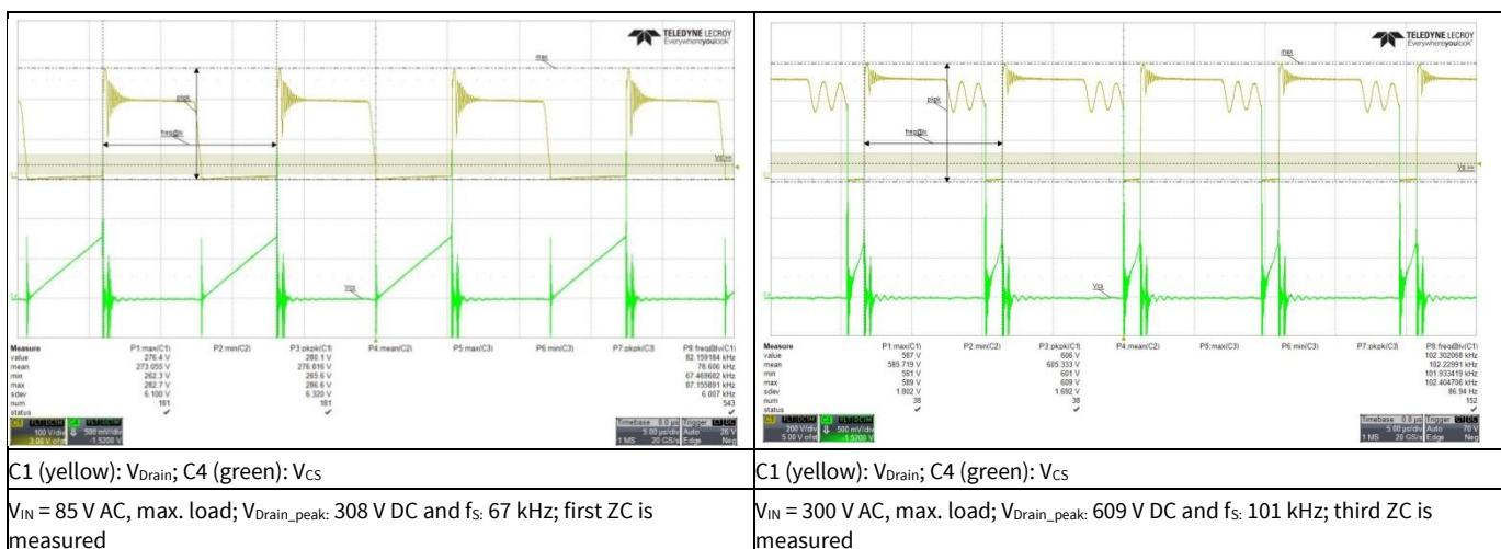
**Figure 16 Drain and CS voltage at maximum load**
