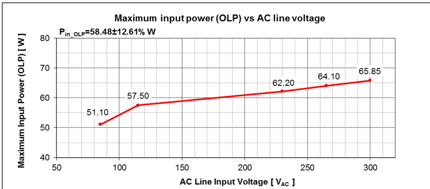
Figure 13 Maximum input power (before over-load protection) vs AC-line input voltage
