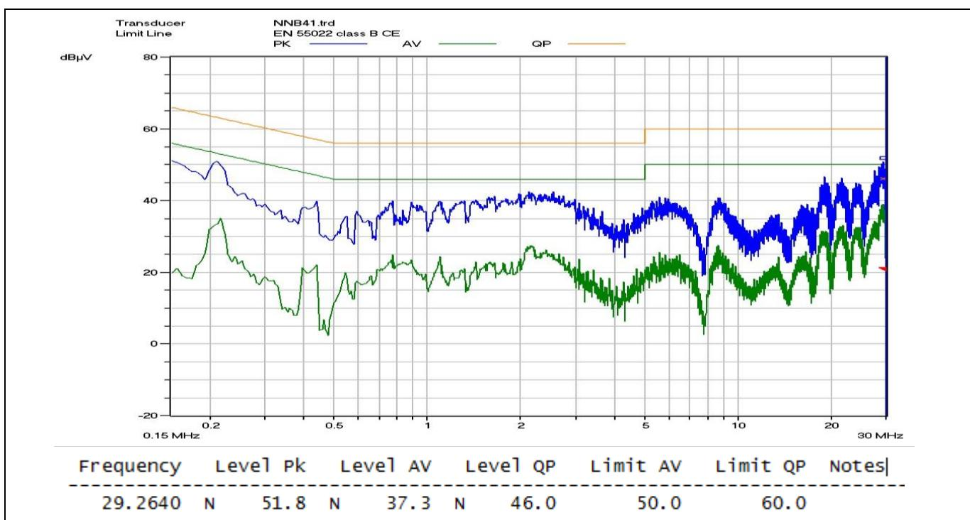
**Figure 26** Conducted emissions at 115 V AC neutral and 33 W load -> 15 dB margin
