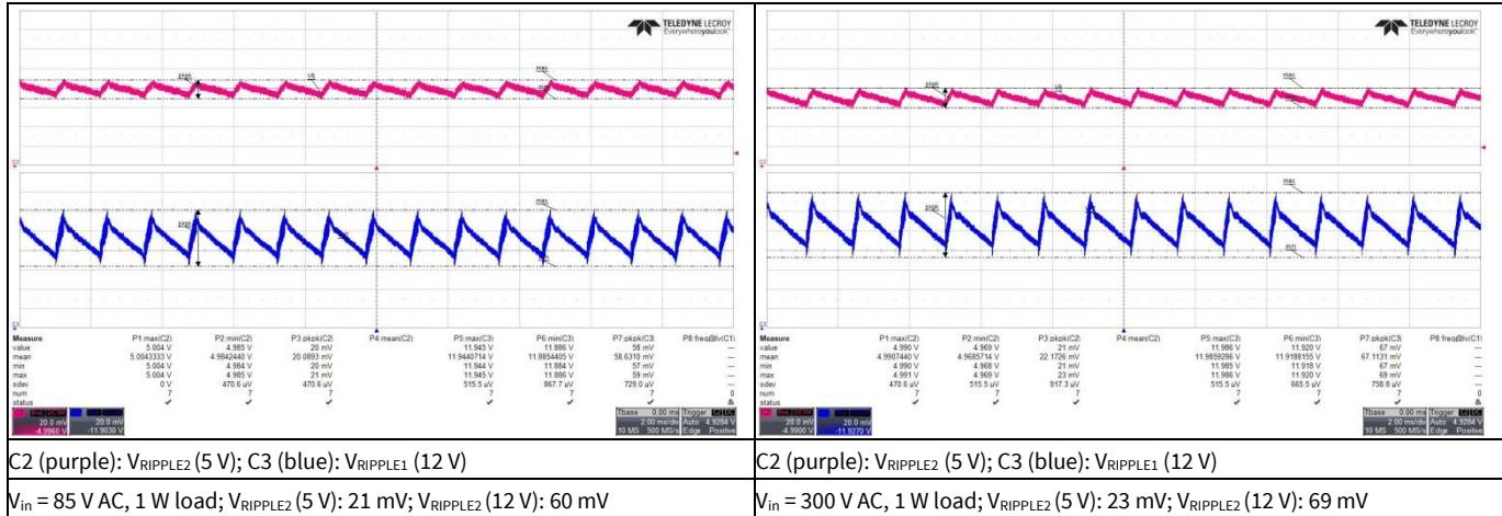
Figure 19 Output ripple voltage in ABM 1 W load
