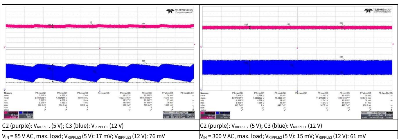
Figure 18 Output ripple voltage at maximum load
