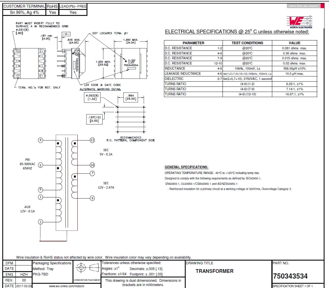
Figure 29 WE transformer specification
