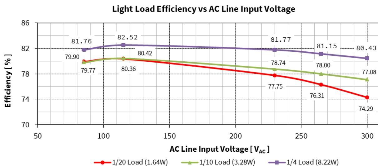
Figure 11 Efficiency vs AC-line input voltage
