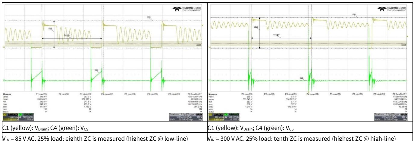
Figure 17 Drain and CS voltage at 25% load
