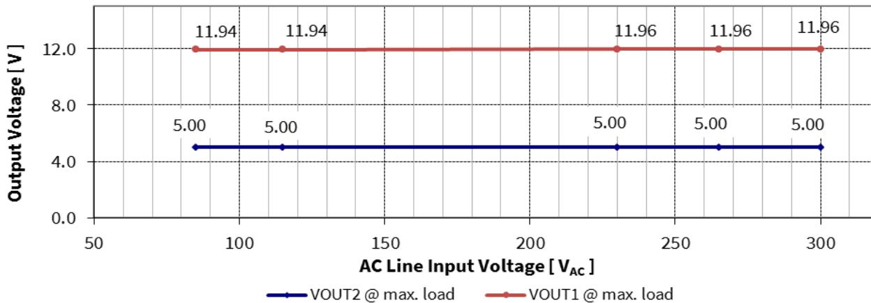
**Line Regulation: Output voltage vs AC line input voltage @ typ. load**
