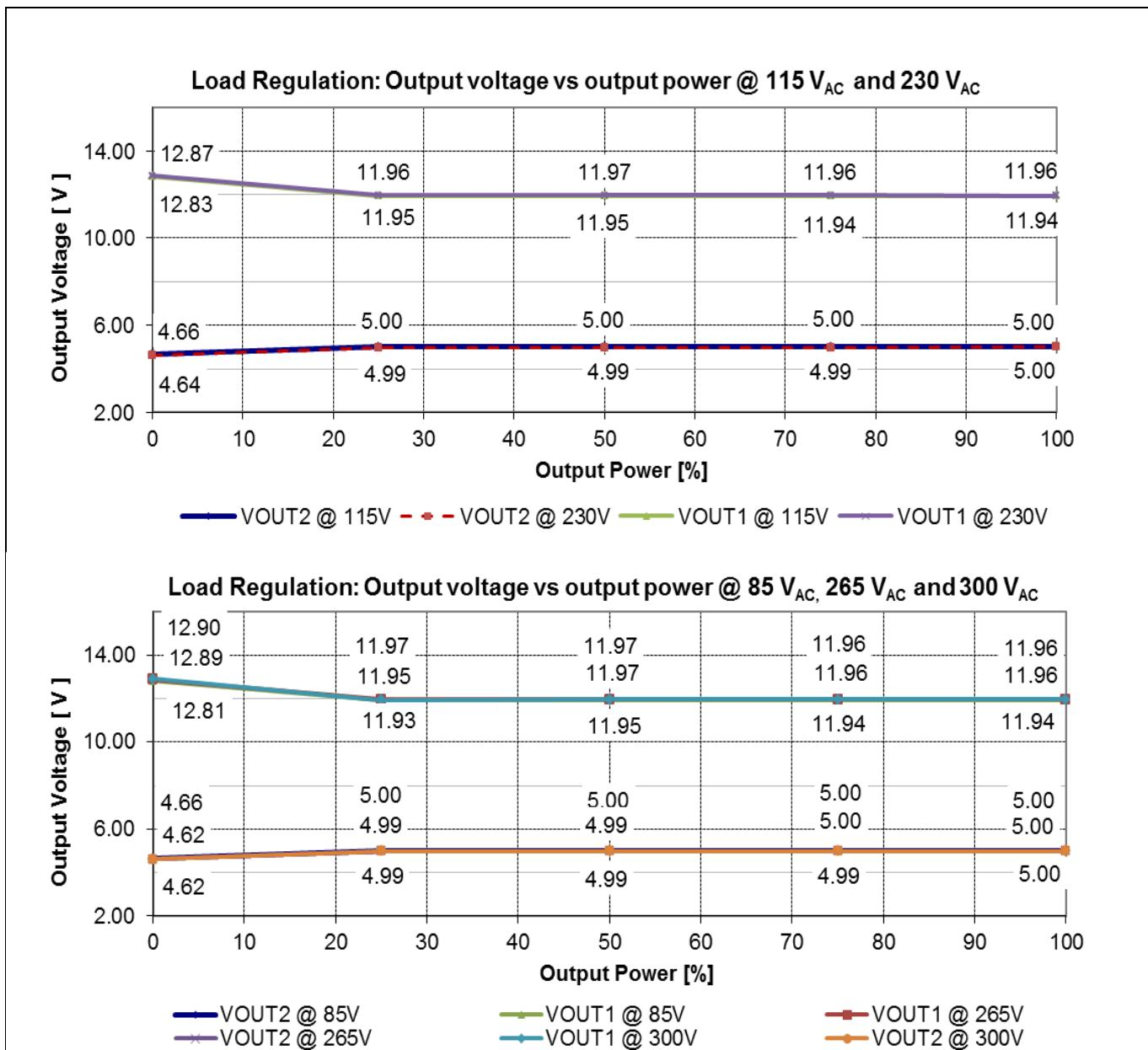
**Figure 9 Load regulation  $V_{\text{OUT}}$  vs output power**
