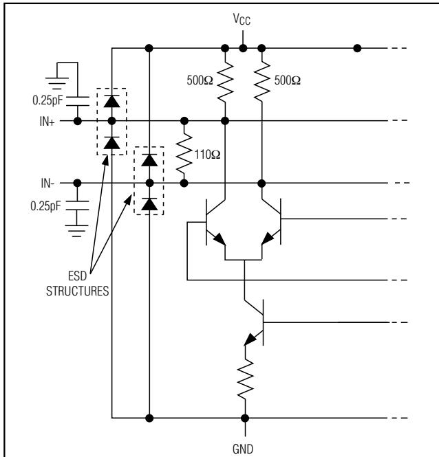
Figure 4. Input Circuit
