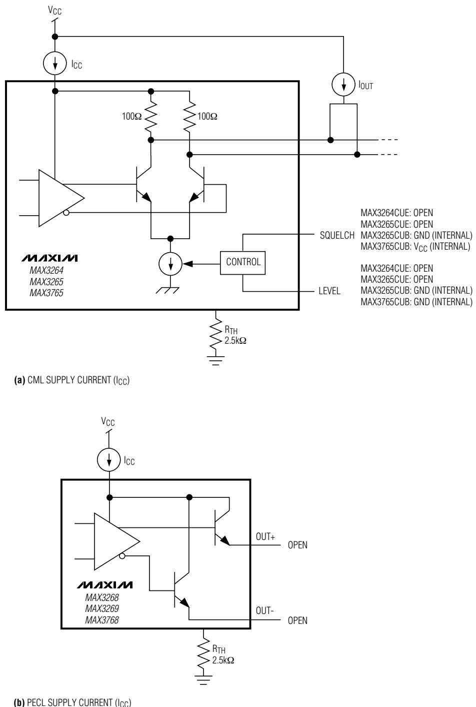
Figure 2. Power-Supply Current Measurement
