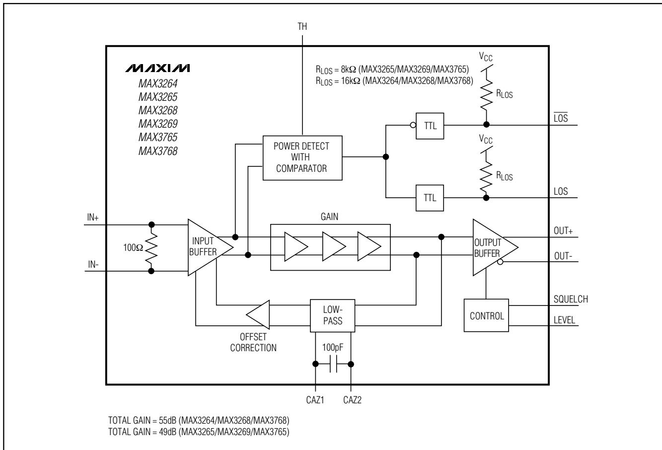
Figure 3. Functional Diagram
