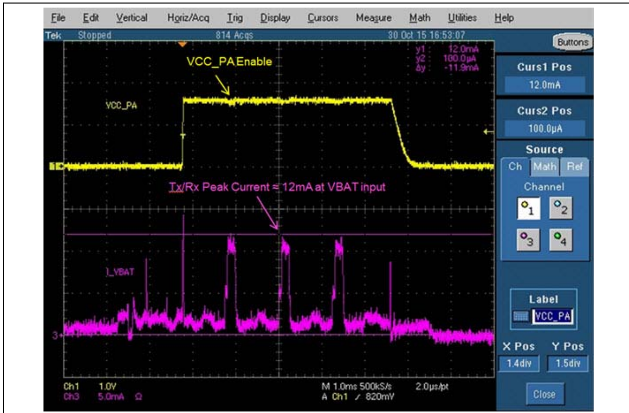
FIGURE 5-1: TX/RX PEAK CURRENT CONSUMPTION OF AN ADVERTISING EVENT
