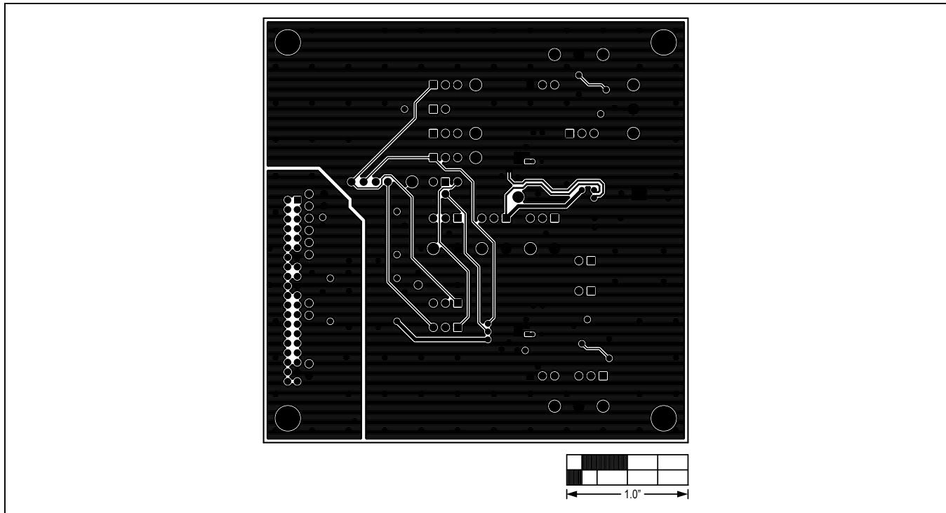
Figure 7. MAX11166 Daughter Board PCB Layout—Solder Side
