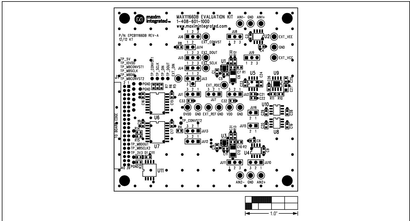
Figure 3. MAX11166 Daughter Board Component Placement Guide—Component Side
