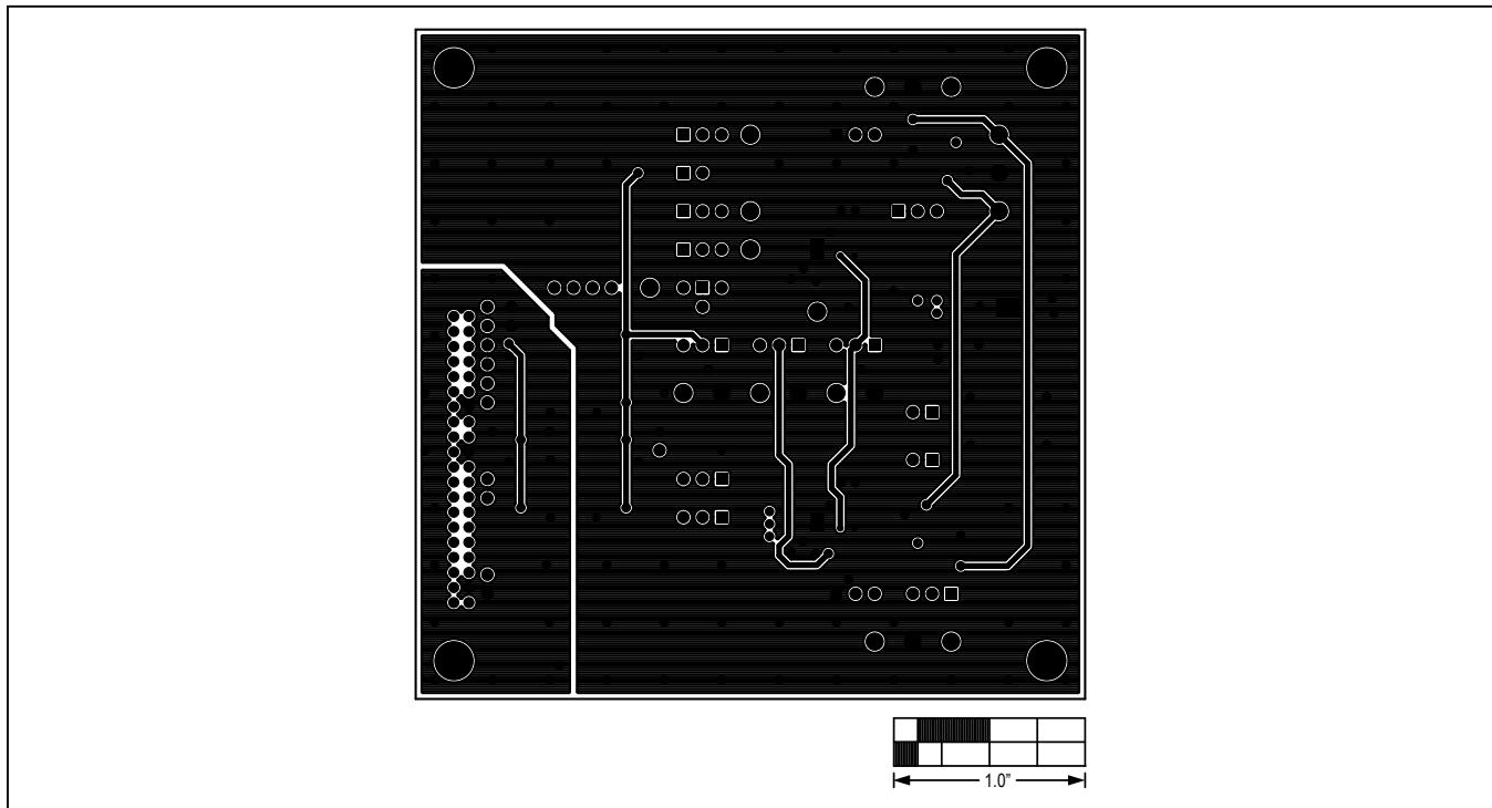
Figure 6. MAX11166 Daughter Board PCB Layout—Power Layer 3
