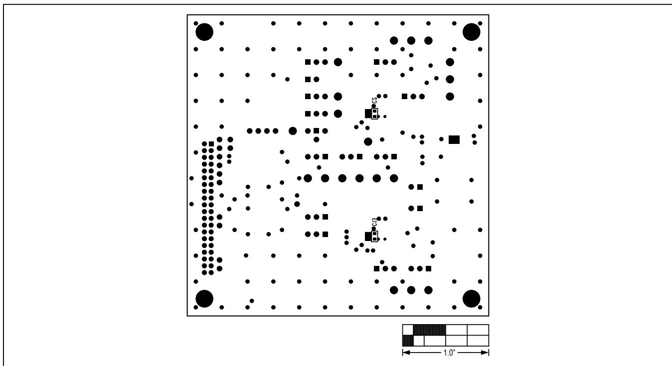
Figure 8. MAX11166 Daughter Board Component Placement Guide—Solder Side
