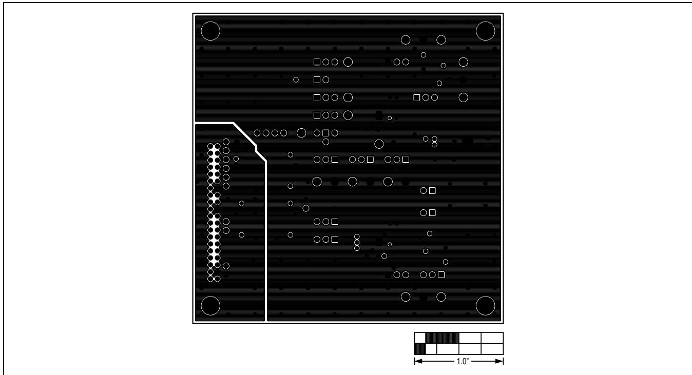
Figure 5. MAX11166 Daughter Board PCB Layout—Ground Layer 2
