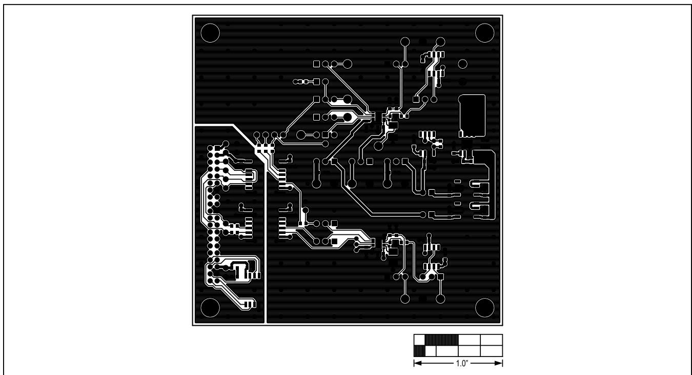
Figure 4. MAX11166 Daughter Board PCB Layout—Component Side
