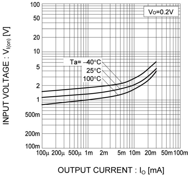
Fig.2 Output Current vs. Input Voltage
