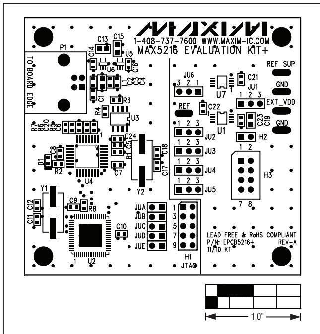
*Figure 6. MAX5216 EV Kit Component Placement Guide—Component Side*
