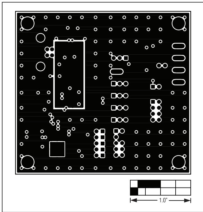
Figure 9. MAX5216 EV Kit PCB Layout—Inner Layer 3
