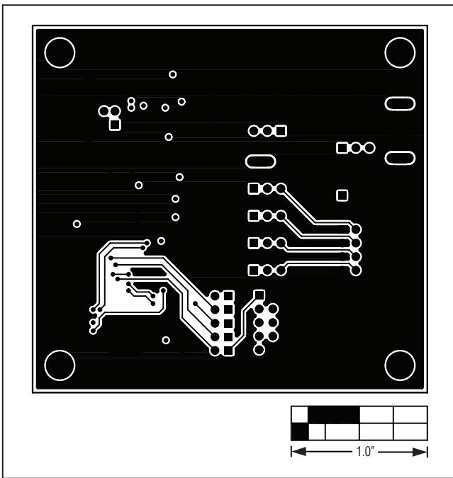
Figure 10. MAX5216 EV Kit PCB Layout—Solder Side
