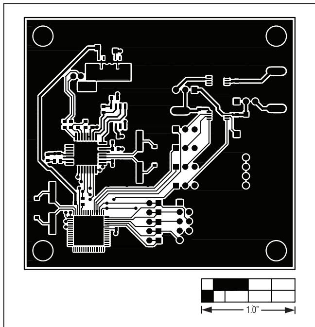
*Figure 7. MAX5216 EV Kit PCB Layout—Component Side*
