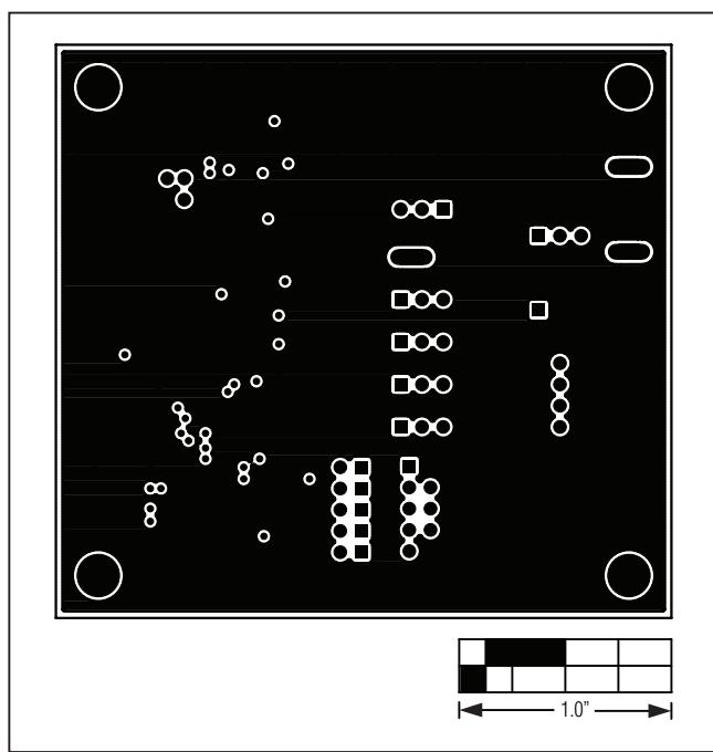
Figure 8. MAX5216 EV Kit PCB Layout—Inner Layer 2
