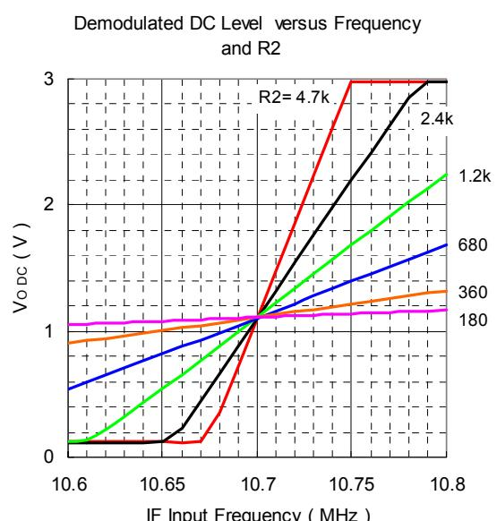
The maximum output level is approximately 90% of supply voltage under the following condition:
