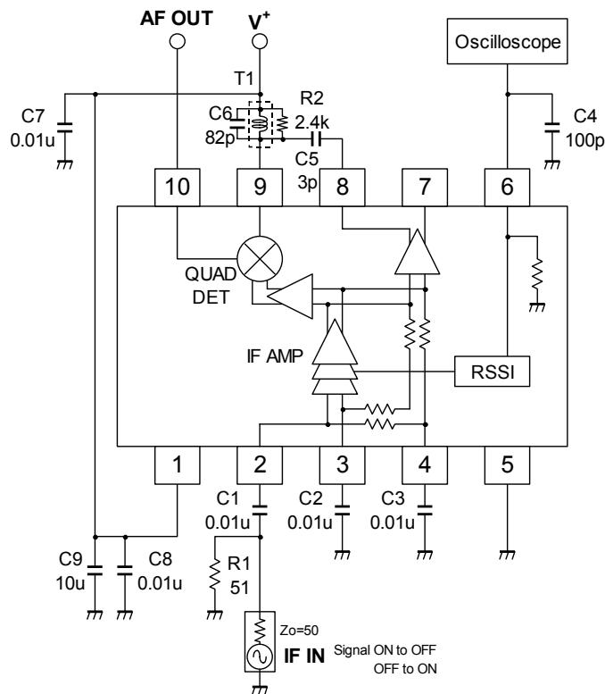
● Test Circuit 8 for Demodulated signal (LPF is connected)
