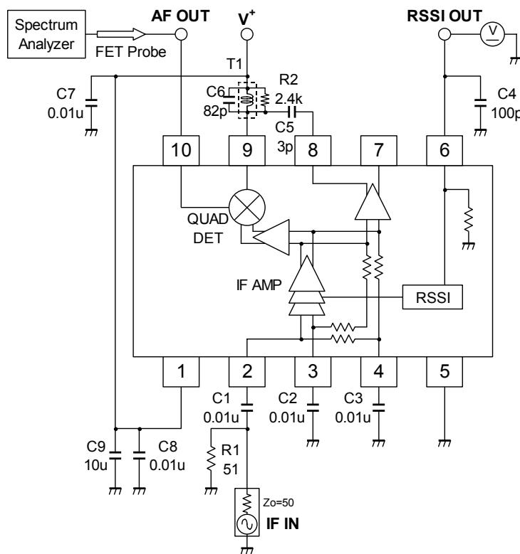
● Test Circuit 6 for Demodulated Signal Frequency Characteristics (Detected Output: N-Curve)
