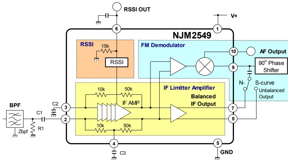
as the same value of the matching impedance. When you connect measurement equipment to Pin2, recommended value of R1 is 50ohm that is the same value of output impedance of the equipment.
