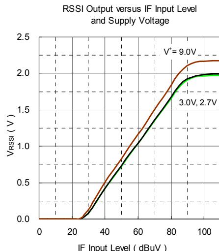
NJM2549 has an internal resistance of 15kohm at Pin6. When  $C_{EXT}=1nF$ , the calculated value of T ( $T1 \rightarrow T2$ ) is 15usec. If another large external capacitance exists, this also influences to the RSSI response time.
