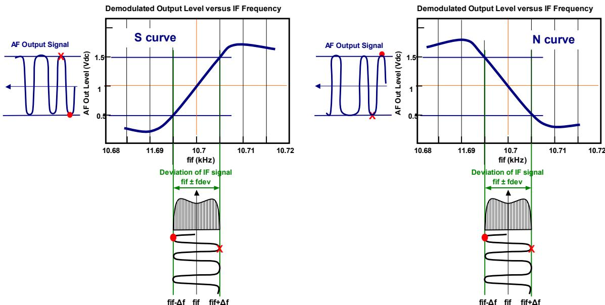
Pin 7 is a select pin for N curve, and pin8 is for S curve. It is recommended that you leave unused pin (Pin7 or Pin8) unconnected on the board, otherwise, terminated with resistor which value is the same as the load impedance of the used pin.
