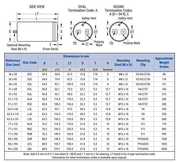
Screw Terminal Aluminum Electrolytic Capacitors - ALS32/33, +85°C
