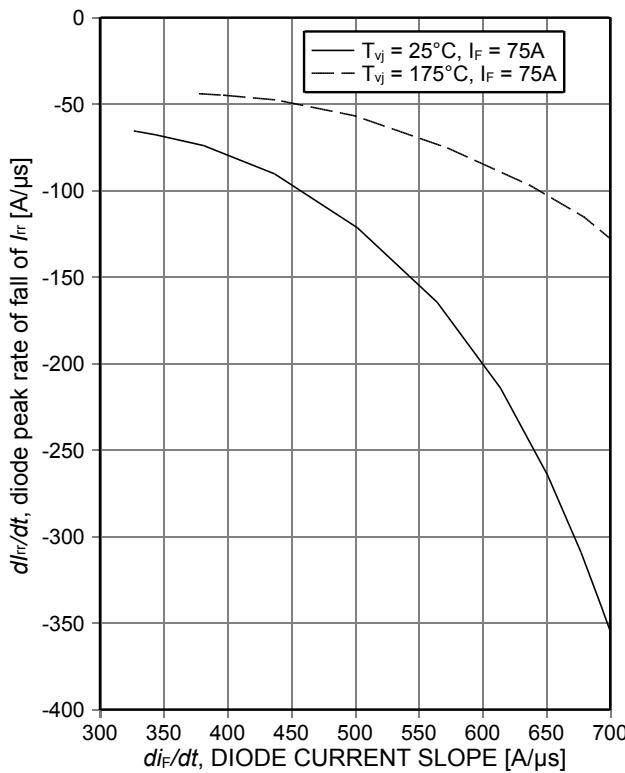
Figure 25. Typical diode peak rate of fall of reverse recovery current as a function of diode current slope
