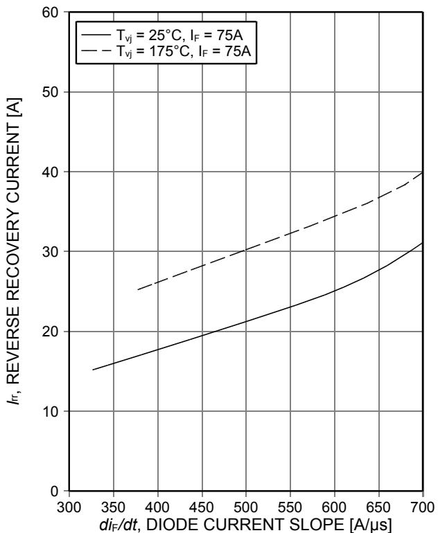
Figure 24. Typical reverse recovery current as a function of diode current slope
