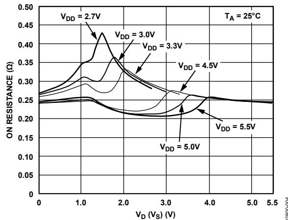
Figure 4. On Resistance vs.  $V_D$  ( $V_S$ )
