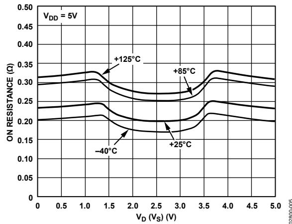
Figure 5. On Resistance vs.  $V_D$  ( $V_S$ ) for Different Temperatures
