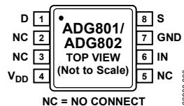
Figure 3. 8-Lead MSOP
