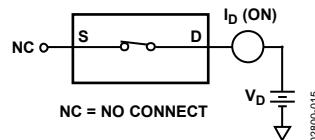
Figure 15. On Leakage
