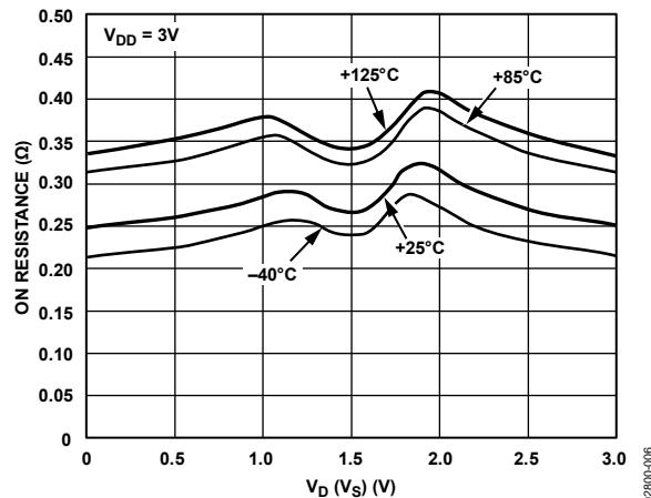
Figure 6. On Resistance vs.  $V_D$  ( $V_S$ ) for Different Temperatures
