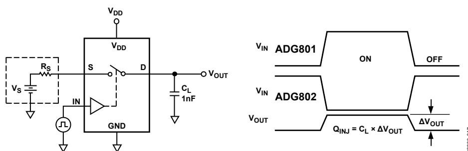
Figure 17. Charge Injection
