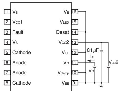
**Fig. 5 VOH Test Circuit**
