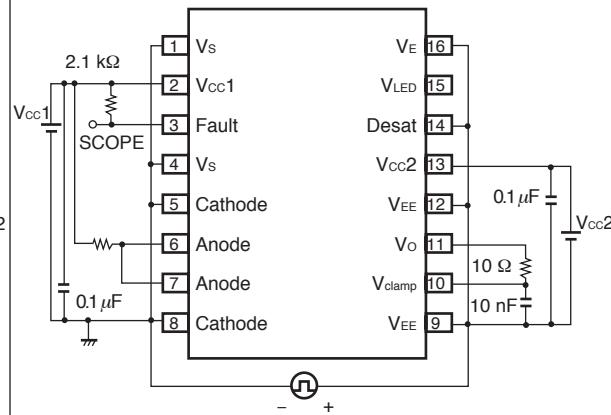
Fig. 23 CM<sub>H</sub>, CM<sub>L</sub> Test Wave Forms (LED1 ON, OFF)
