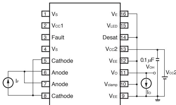
**Fig. 6 VOL Test Circuit**
