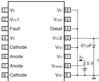
**Fig. 12  $V_{DESAT}$  Test Circuit**
