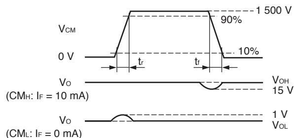
Fig. 24 CM<sub>H</sub>, CM<sub>L</sub> Test Wave Forms (LED2 ON, OFF)
