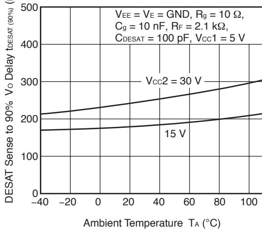
DESAT SENSE TO 10%  $V_O$  DELAY vs. AMBIENT TEMPERATURE
