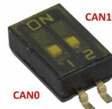
Figure 44: CAN Termination Switch
