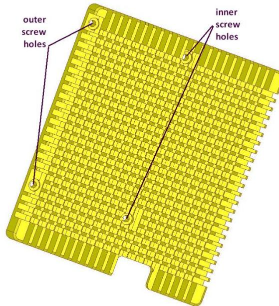
For the removal of the module, first unplug all connections to the system. Take off the inner screws, then the outer ones. The thermal pad may cause the heatsink sticking to the module, so take care, while pulling apart to avoid collisions with any part of the module. Lift the module to about 25°and remove it from the connector. Store the parts on a static free area.
