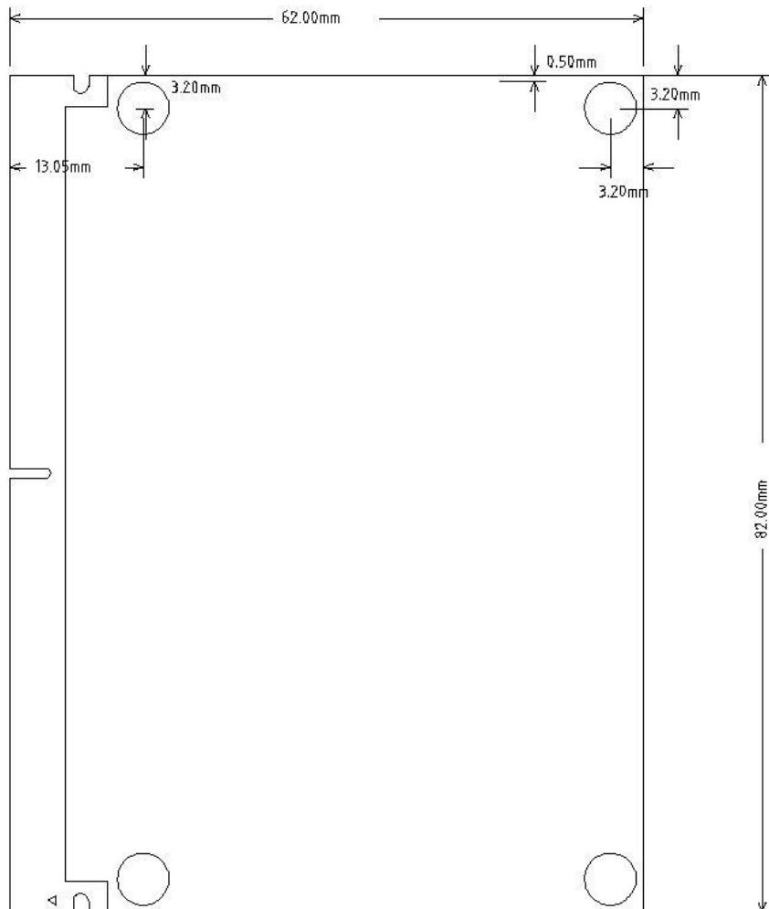
Figure 8 Mechanical Dimensions
