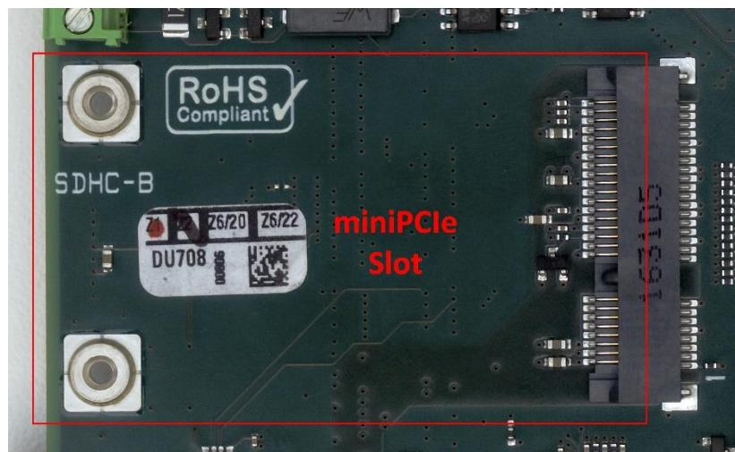
Figure 33: miniPCIe Slot
