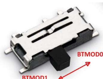
Shown positions set the according BTMOD0/1 line to low. BTMOD0 controls the CPU configuration port PC9, i.e. BOOTMOD(0), while BTMOD1 is connected to the CPU configuration port PC10, i.e. BOOTMOD(1).
