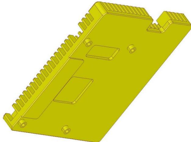
Insert the outer screws first and tighten them just a few turns. Then insert the two inner screws also with a few turns. Now check the gap between carrier and module for other parts than the CPU touching the heatsink. Check the thermal CPU pad for correct position. Tighten the four screws with no more than 30Ncm.
