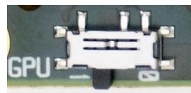
Figure 25: GPU Power On (default)
