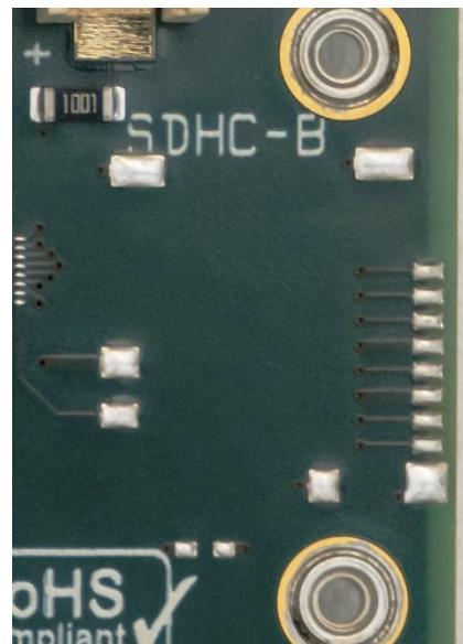
Figure 39: not fitted SDHC-B connector
