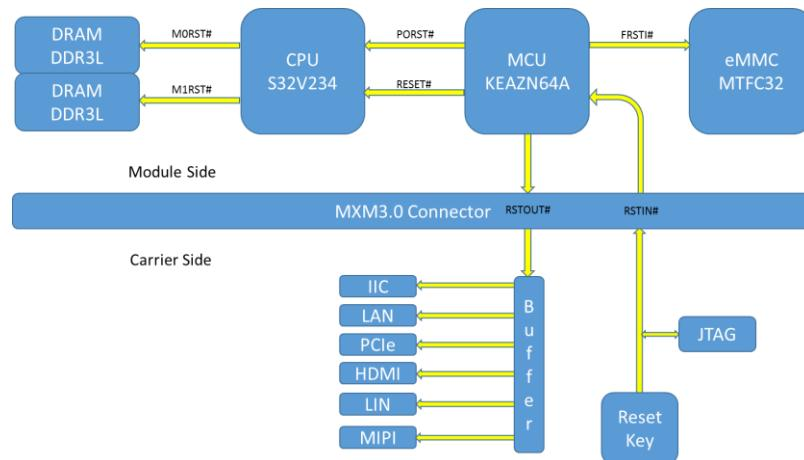
Figure 4-3 Reset Structure
