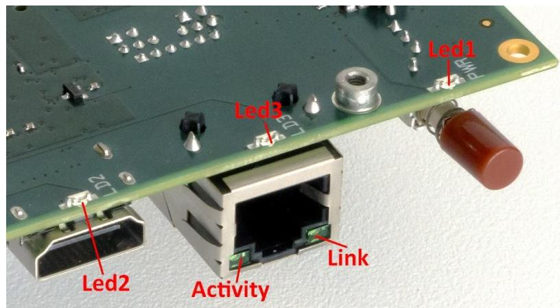
Figure 45: Carrier LEDs
