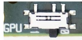
Figure 24: GPU Power Off
