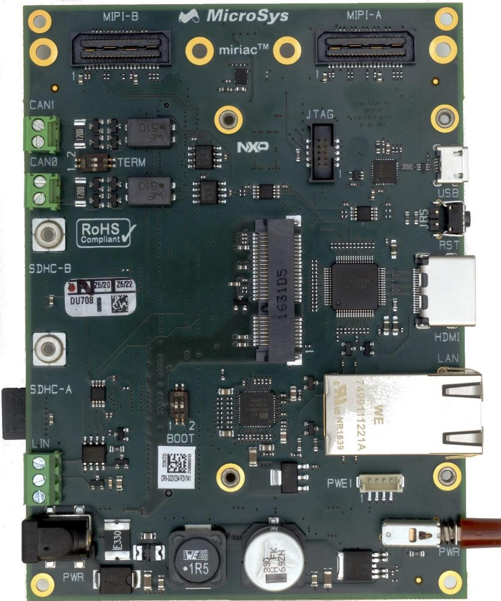
Figure 10 Non-Module Side connectors (carrier CRX-S32V)
