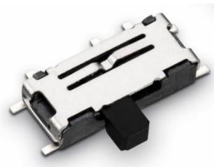
The CAN termination switch is used to enable or disable a 120R termination resistor for each CAN line. For more information refer to **9.7.3 Termination**
