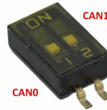
Figure 44: CAN Termination Switch
