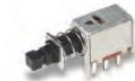
The boot mode switch is used to select between 4 possible boot configurations, implemented in the MCU. For more information refer to [5.3 Boot Mode Switch](#) and [5.2 Power Up Configuration](#)
