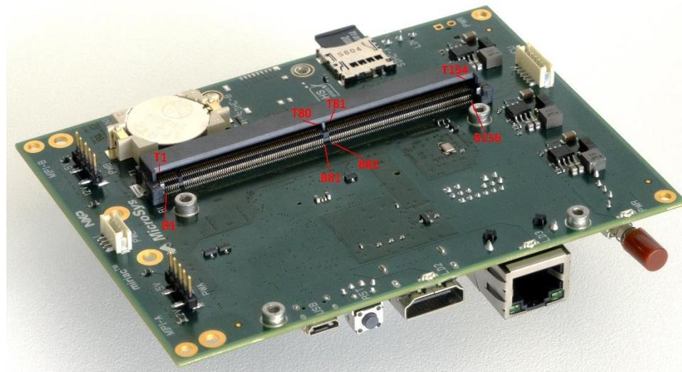
Figure 27: MXM-Connector
