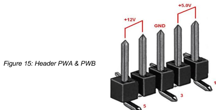
Figure 15: Header PWA & PWB
