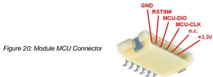
Figure 20: Module MCU Connector
