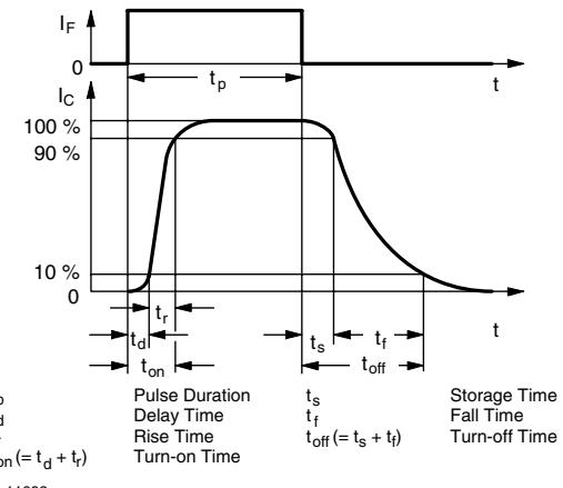
Fig. 3 - Switching Times
