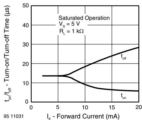
Fig. 12 - Turn-on/off Time vs. Forward Current
