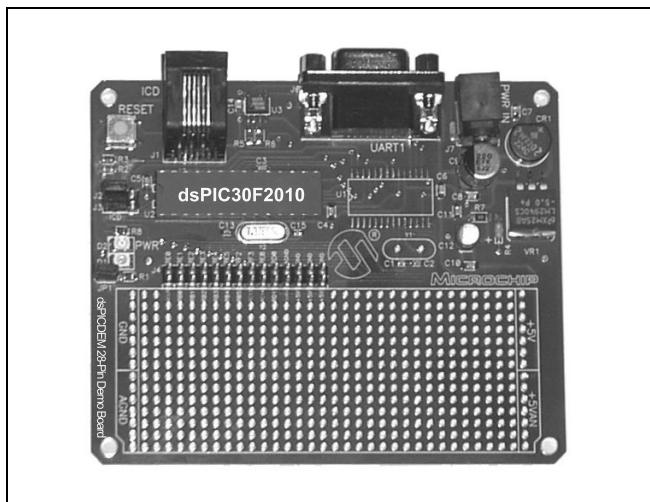
The low-cost dsPICDEM 28-Pin Starter Development Board allows the user to easily validate a development tool setup using a 28-pin SDIP or SOIC dsPIC30F device. The development board has a socketed dsPIC30F2010 digital signal controller, power supply regulator, crystal oscillator, MPLAB® ICD header, serial port, power-on indicator, Reset push button, 28L SOIC layout pad and a prototyping area.
