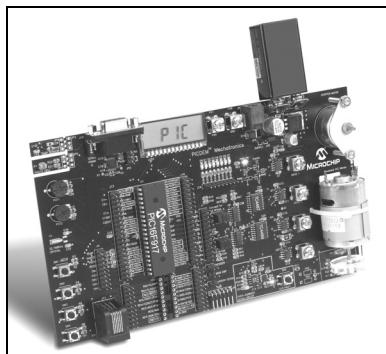
The PICDEM Mechatronics Demonstration Kit is an easy-to-use mechatronics development and demonstration platform. Mechatronics refers to implementing intelligent control in a mechanical system. Learn how to use PIC® microcontrollers to enhance or replace a mechanical design.
