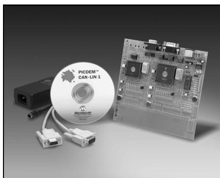
Microchip offers three similar PICDEM CAN-LIN Demonstration Boards to support different PICmicro® devices. All demonstrate the main features of the
