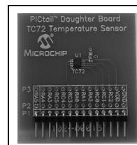
Connects directly to the PICkit 1 Flash Starter Kit. Highly accurate board features a 10-bit digital sensor with 3-wire SPI™ interface.
