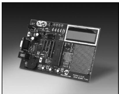
The PICDEM 2 Plus Demonstration Board is a powerful, low-cost learning and demonstration board. The board comes with an active program loaded on the installed
