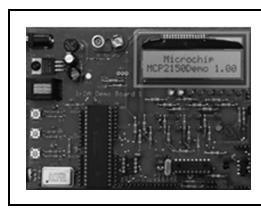
Includes everything needed to create a system that uses infrared to communicate. Kit contains two MCP2120 developer's boards and one MCP2150 developer's board.
