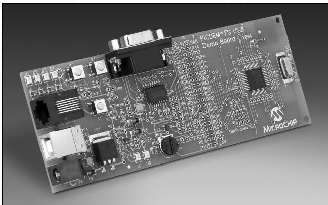
The PICDEM™ FS USB is a demonstration and evaluation board for the PIC18F4550 family of Flash microcontrollers with Full-Speed USB 2.0 interface. The board contains a PIC18F4550 microcontroller in a 44-pin TQFP package, representing the superset of the entire family of devices offering the following features:
