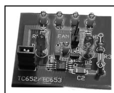
Allows users to quickly prototype fan control circuits on TC652 or TC653 PWM fan control ICs. The board can interface with virtually any brushless DC fan.
