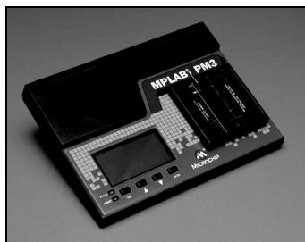
The MPLAB PM3 Universal Device Programmer is easy-to-use and operates with a PC or as a stand-alone unit, and programs Microchip's entire line of PICmicro® devices, as well as the latest dsPIC30F DSC devices. The MPLAB PM3 features a large and bright LCD unit (128 x 64 pixels) to display easy menus, programming statistics and status information.
