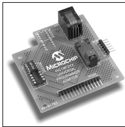
The PIC10F2XX Universal Programmer Adapter provides PIC10F socket support for both the SOT-23 and DIP-8 packages. It allows interfacing to Microchip's low-cost family of programmers, inclusive of:
