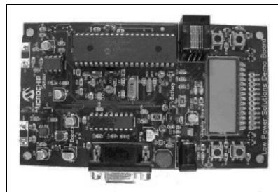
The Low-Power Solutions Demonstration Board provides designers a convenient and fun way to explore PICmicro® MCU nanoWatt features
