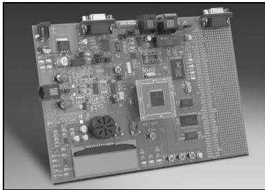
The dsPICDEM.net 1 and dsPICDEM.net 2 Connectivity Development Boards provide the application developer a basic platform for developing and evaluating both connectivity and non-connectivity-based requirements.
