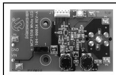
Demonstrates the MCP165X Boost Controller product family in a battery-powered white LED application with an input voltage range of 2.0V to 4.5V.
