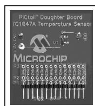
Demonstrates how to interface the TC1047A device to a microcontroller. Connects directly to the PICkit 1 Flash Starter Kit, providing a platform for code development and evaluation. Provides a good example of how to integrate an analog temperature sensor into a system.
