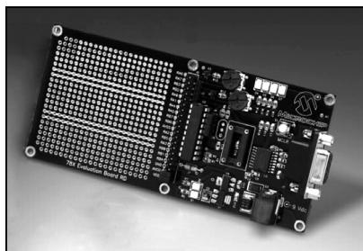
The PICDEM MSC1 Demonstration Kit with its PC-based Graphical User Interface (GUI) software serves as a demonstration board for the PIC16C781/782
