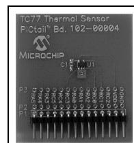
System designers can use this design as an example of how to integrate a digital temperature sensor into their systems. Connects directly to the PICkit 1 Flash Starter Kit.
