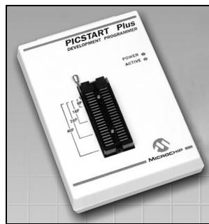
The PICSTART Plus Programmer gives the product developer the ability to program user software into any of the supported microcontrollers. The PICSTART Plus Programmer software, running under MPLAB® IDE, provides for full interactive control over the programmer.
