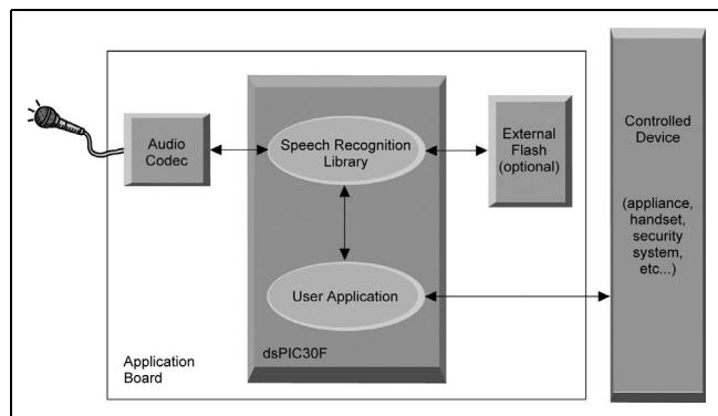
The Speech Recognition Library provides isolated, speaker-independent word recognition of US English. It allows the user to control an application through a set of fixed, voice commands.
