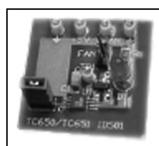
Allows users to quickly prototype fan control circuits based on the TC650 or TC651 PWM fan control ICs.
