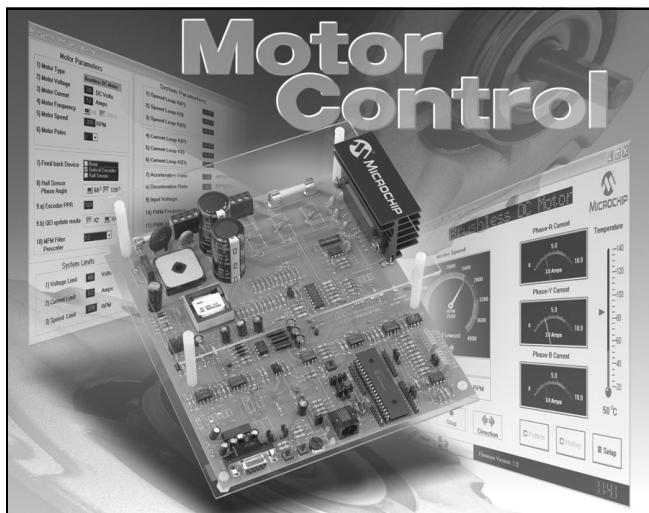
The PICDEM MC Development Board provides designers with a quick method to evaluate and develop both AC and DC motor control applications utilizing Microchip's family of 28 and 40-pin enhanced microcontrollers. The development board is ideal for beginning motor control designers, as well as those new to the PIC18F2331/2431/4331/4431 family of motor control devices.
