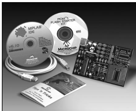
The PICkit 1 Flash Starter Kit is a low-cost development kit with an easy-to-use interface for programming Microchip's 8/14-pin Flash family of microcontrollers. This starter kit is
