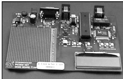
The PICDEM.net Demonstration Board is an Internet/Ethernet demonstration board using the PIC18F452 microcontroller and TCP/IP
