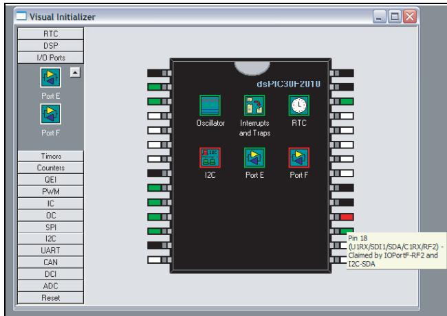
Microchip's MPLAB IDE Visual Device Initializer allows users to configure Microchip microcontrollers graphically, and when configuration is complete, a mouse click generates code usable in Assembly or 'C' programs.
