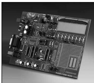
The PICDEM 4 Demonstration Board supports Microchip's low pin count PICmicro® Flash microcontrollers, including the PIC16F and PIC18F families featuring nanoWatt Technology. nanoWatt Technology
