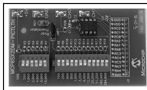
Features MCP6S22 and MCP6S92 PGAs. Helps overcome nonlinear response of the on-board NTC thermistor. Opens possibilities of temperature correcting another sensor and increasing the number of PIC microcontroller I/O pins available for other purposes.
