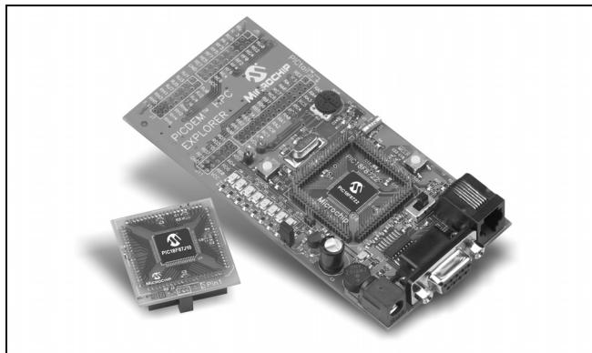
The PICDEM HPC Explorer Board is the latest 64/80 TQFP demonstration board for evaluating Microchip Technology's PIC18F and PIC18FXXJXX families of devices. It comes populated with a PIC18F8722 MCU. Direct connection support is available for the MPLAB® ICE 2000 and MPLAB ICE 4000 processor modules, plug-in modules and MPLAB ICD 2 In-Circuit Programmer.
