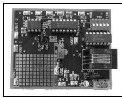
Provides a versatile selection of input channels and gains to evaluate device performance. Board supports multiple input signal sources. Two devices can be cascaded to produce gain to 1024 V/V.
