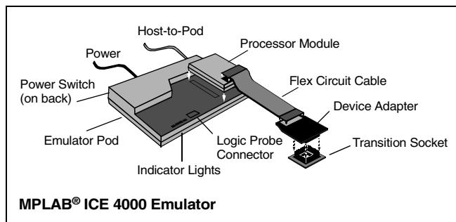
An MPLAB ICE emulator system is ordered as separate components. Knowing the terms will make it easy to order and use the MPLAB ICE emulator system. Read more about each component.
