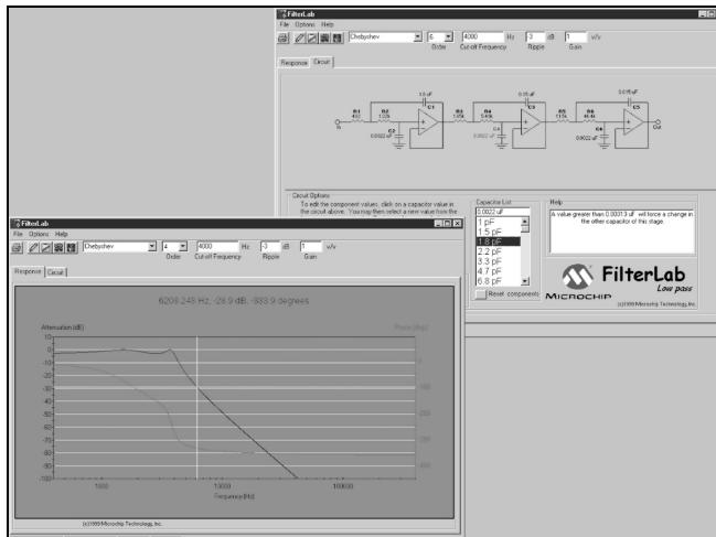
FilterLab Active Filter Software Design Tool is an innovative software tool that simplifies active filter design. The FilterLab Active Filter Software Design Tool provides full schematic diagrams of the filter circuit with component values and displays the frequency response.
