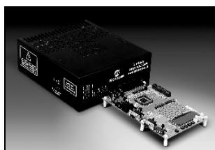
The MC1 Motor Control Development Board provides the application developer with three main components for quick prototyping and validation of BLDC, PMAC and ACIM applications. The three main components are: dsPIC30F motor control main board, 3-phase, low-voltage power module and 3-phase, high-voltage power module.
