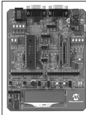
The dsPICDEM™ 2 Development Board is a development and evaluation tool that helps you create embedded applications using dsPIC30F Digital Signal Controllers. Sockets are provided for 28 and 40-pin devices in the motor control family and 18, 28 and 40-pin devices in the general purpose and sensor family. The supported
