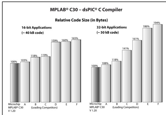
The MPLAB C30 C Compiler is a fully ANSI-compliant product with standard libraries for the dsPIC® DSC architecture. It is highly optimizing and takes advantage of many dsPIC DSC architecture-specific features to provide efficient software code generation. MPLAB C30 also provides extensions that allow for excellent support of the hardware, such as interrupts and peripherals. It is fully integrated with the MPLAB IDE for high-level source debugging.
