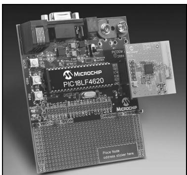
The PICDEM™ Z Demonstration Kit is an easy-to-use ZigBee™ technology wireless communication protocol development and demonstration platform. The demonstration kit includes the ZigBee protocol stack and two
