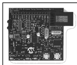
Demonstrates the MCP2140 device in a real-world application. Shows how to integrate an IrDA® standard port.
