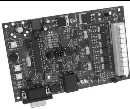
The PICDEM MC LV Development Board provides a cost-effective method of evaluating and developing Sensored or Sensorless Brushless DC
