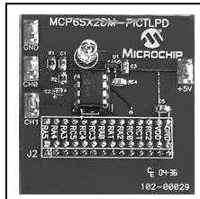
Opens possibilities to process other sensor signals. Increases the number of PIC® microcontroller I/O pins available for other purposes. Features a PNZ334 photodiode, MCP6001U op amp and MCP6S22 and MCP6S92 Programmable Gain Amplifiers (PGA).
