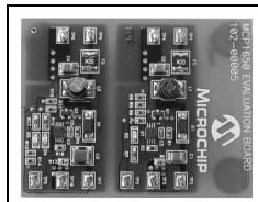
Demonstrates the MCP165X Boost Controller product family in two high-power, boost converter applications.
