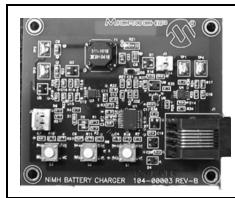
High-speed PWM interfaces to PIC16LF818, providing a complete NiMH battery charger with fuel gauge capability. Minimizes external inductor/capacitor cost. Performs complex NiMH battery charger timing functions. Protects battery circuit if a Fault occurs.
