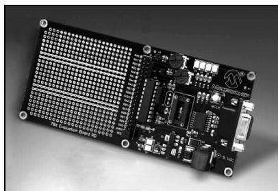
The PICDEM MSC1 Demonstration Kit with its PC-based Graphical User Interface (GUI) software serves as a demonstration board for the PIC16C781/782
