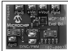
For both battery-powered and distributed-power applications. Operates over a 2.7V to 5.5V input range while delivering 500 mA of output current.
