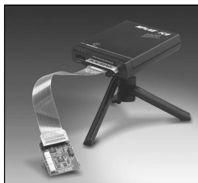
Microchip's universal MPLAB ICE 2000 for PICmicro® MCUs has been designed with user requirements in mind. The system is small, portable, lightweight and offers improved
