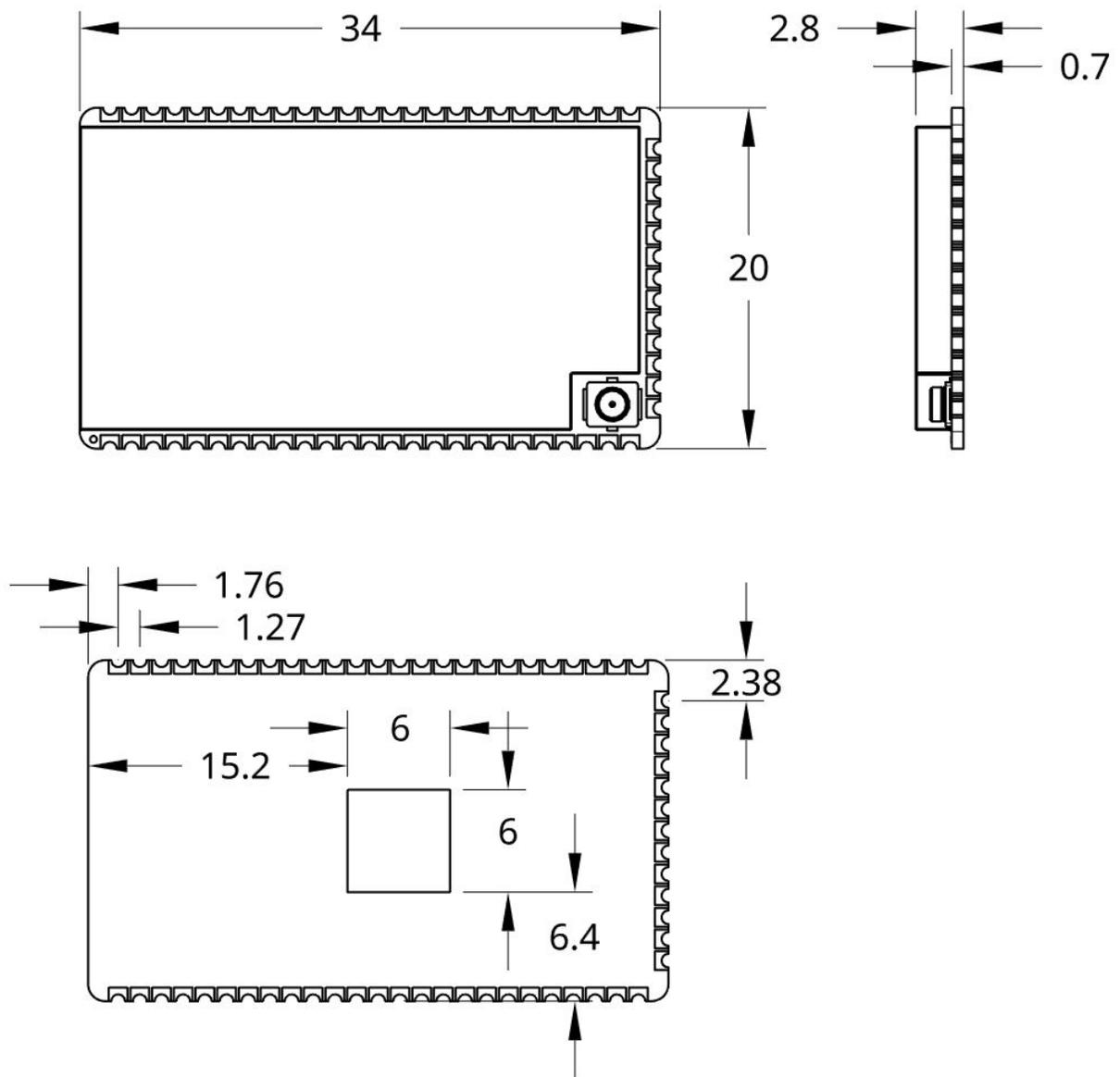
\* All measurements in millimeters
