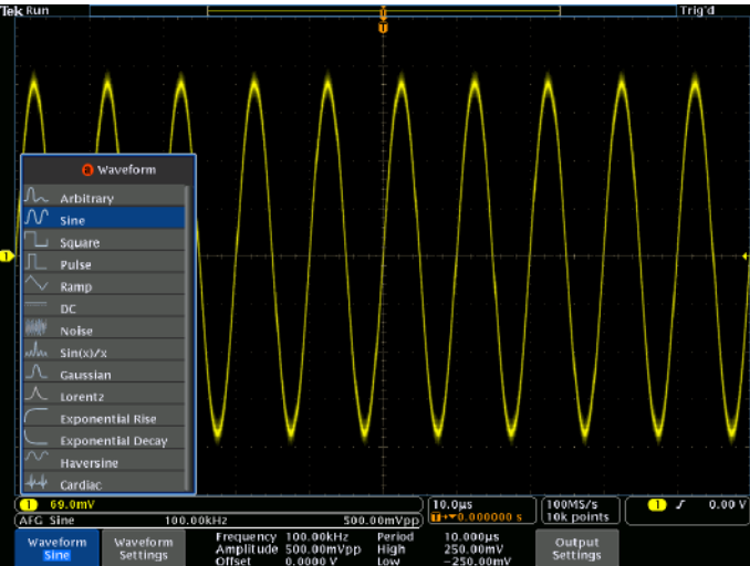
Waveform type selection in the integrated AFG.
